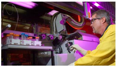
A lab employee performs technical oversight of an Inductively Coupled Plasma-Mass Spectrometer.
