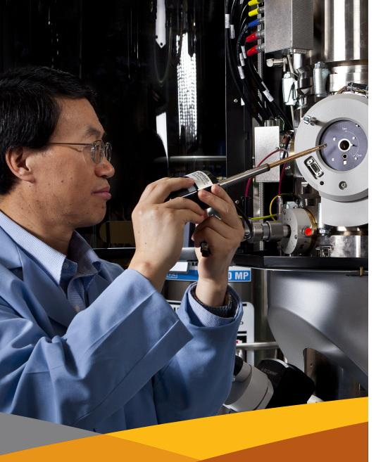
A scientist loads a sample into an aberrationcorrected scanning transmission electron microscope at EMSL. This state-of-the-art instrument enables high-resolution imaging of structural and chemical information for nanomaterials, catalysts, and minerals, and will help in the design of new materials for energy production and storage.
