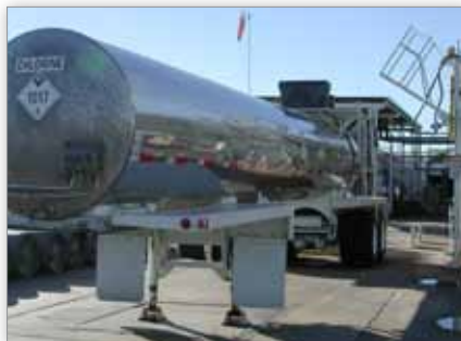
Tanks like this can contain as much as 9,000 gallons of toxic material.
