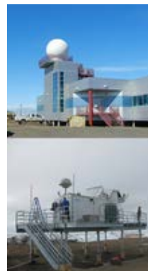
X-band radar on Barrow Arctic Research Center and Vaisala autosonde balloon launcher at ARM's Barrow site.
