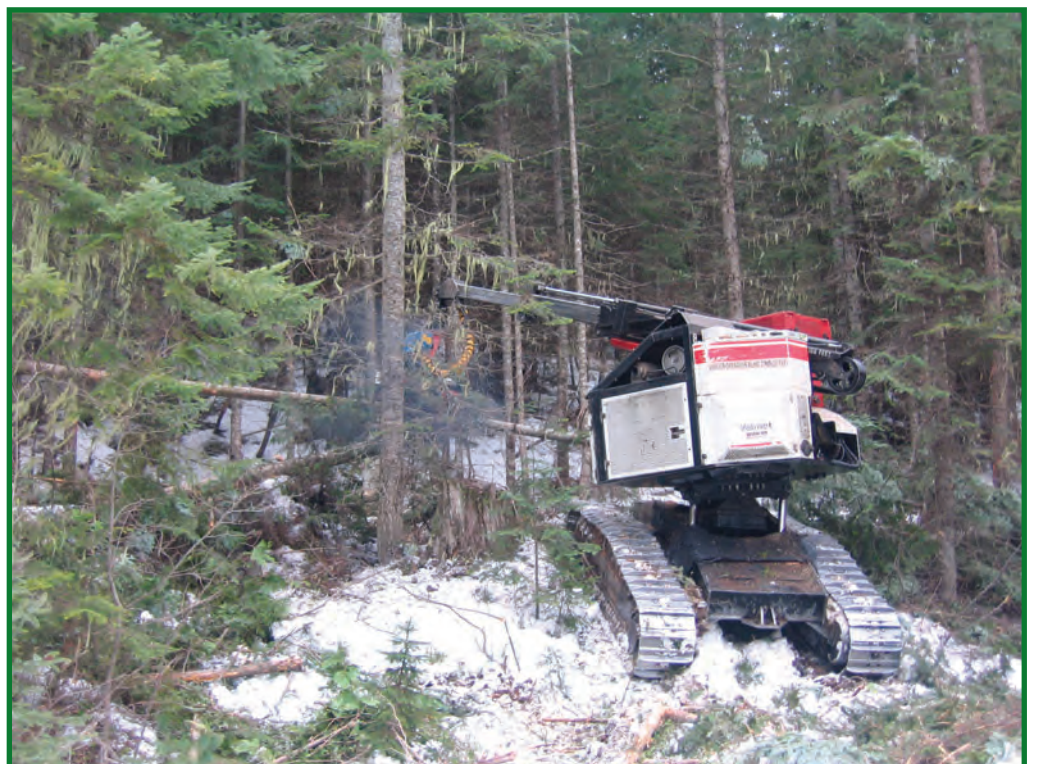
Figure 8.14. Harvester felling and processing trees at the stump, leaving limbs and tops on site.
