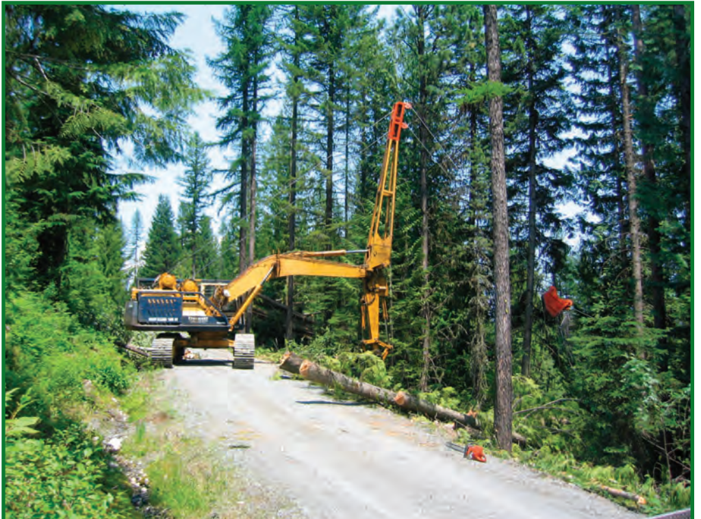
Figure 8.16. An excavator-based yarder performing a fuel reduction thinning in northern Idaho.
