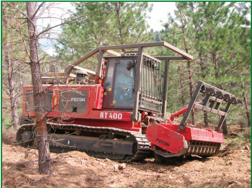
Figure 8.10. Horizontal drum masticator effectively masticating a blanket of shrubs.
