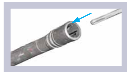
Shove rod into barrel to clear jammed cartridge.
