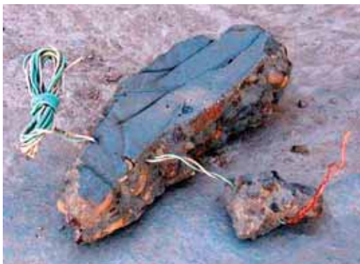
Remote control receiver hidden in plaster.
