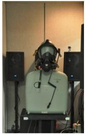
A simulator is set up in a sound isolation booth and used to prepare sound clips for subjective testing.
