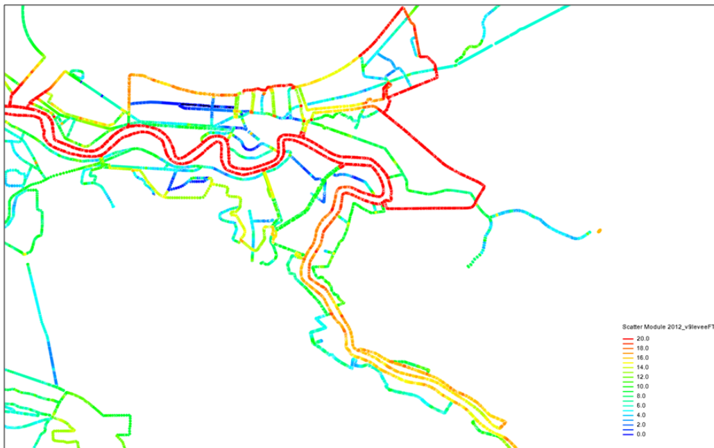
Figure 6.7 Elevations of levees, road systems and other structures represented as sub-grid scale features in the 2012 100-Year HSDRRS condition ADCIRC grid
