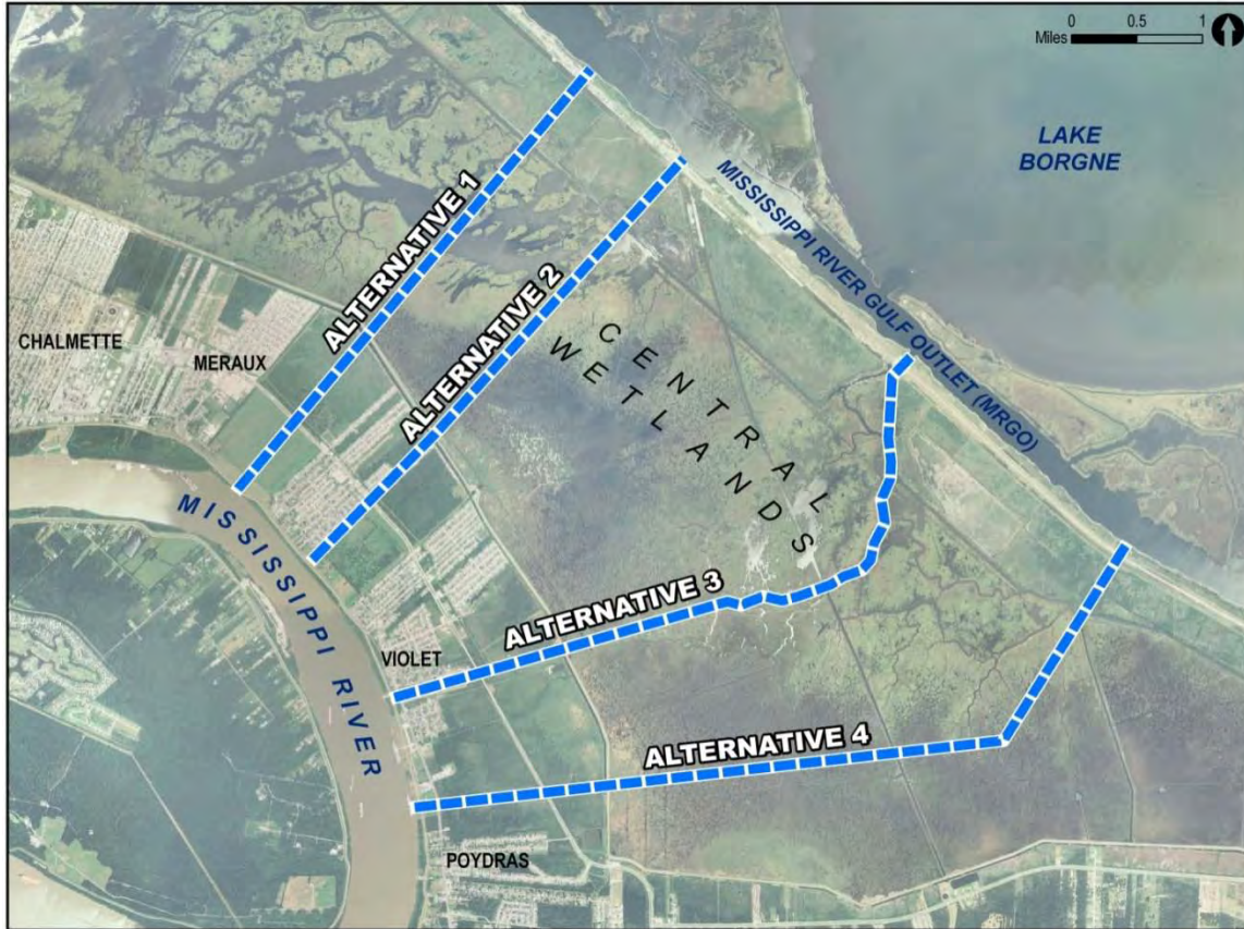
Figure 2-12: Alternative Locations for the Violet, Louisiana Freshwater Diversion Considered in Initial Analysis
