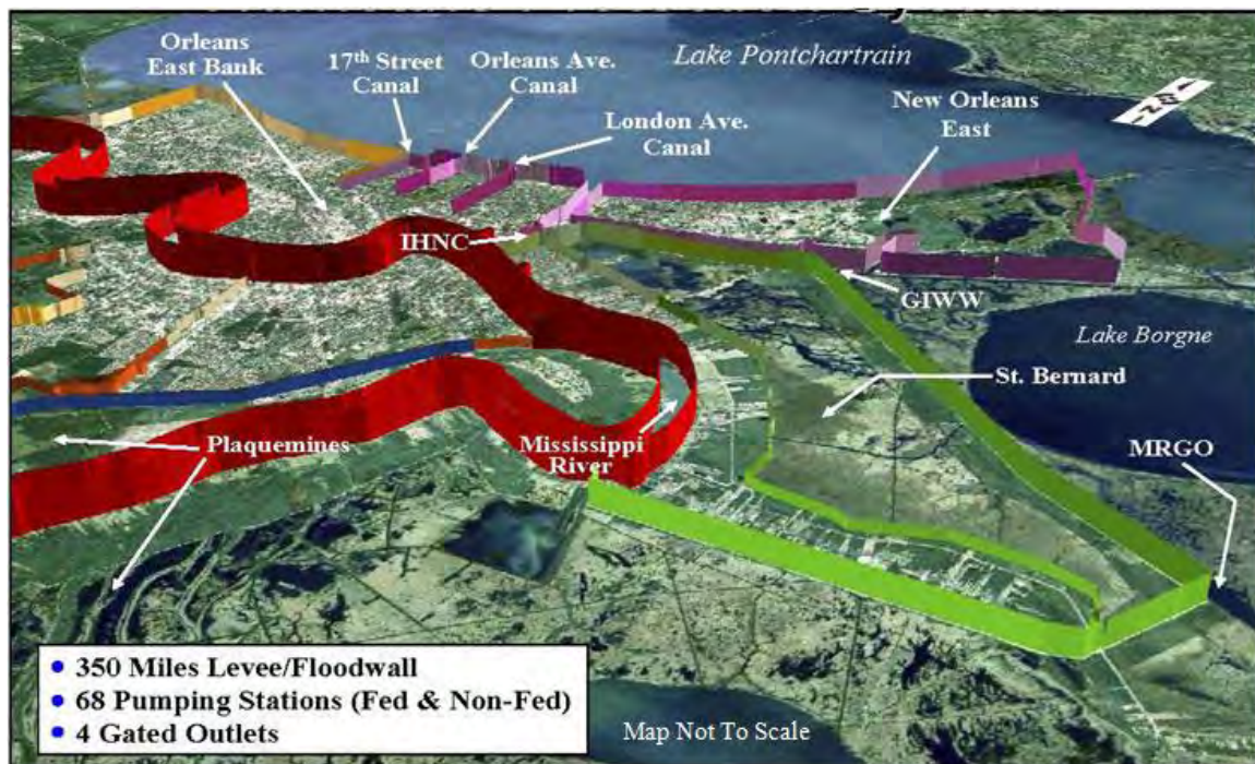
Figure 3-22: Flood Protection Features near the Project Area
