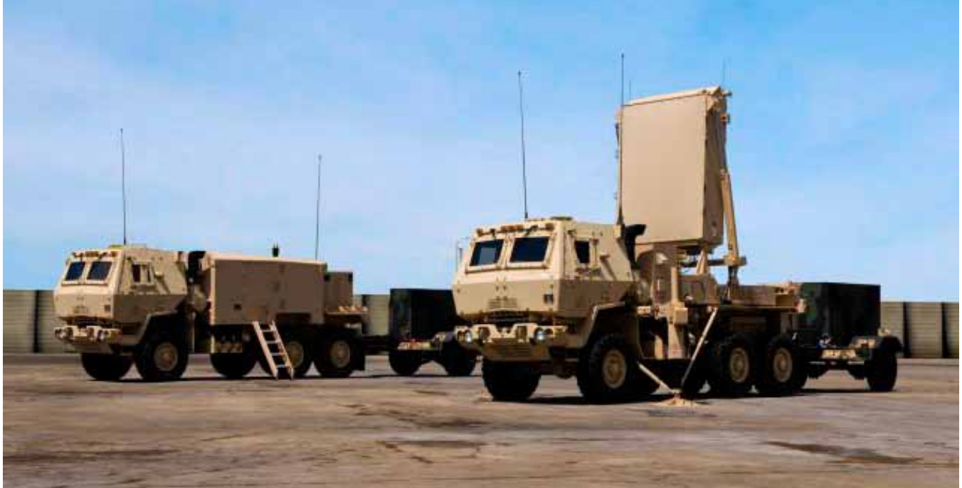
The AN/TPQ-53 Counterfire Target Acquisition Radar provides long-range counterfire target acquisition for mortars, rockets and cannons. Product Manager Radars and Lockheed Martin were recently awarded an excellence in systems engineering award by the Defense Department for their work with AN/TPQ-53. U.S. Army RDECOM CERDEC systems engineers and quality assurance engineers supported the Q-53 radar system and developed the predecessor system prior to it being transitioned to the PM. U.S. Army photo
