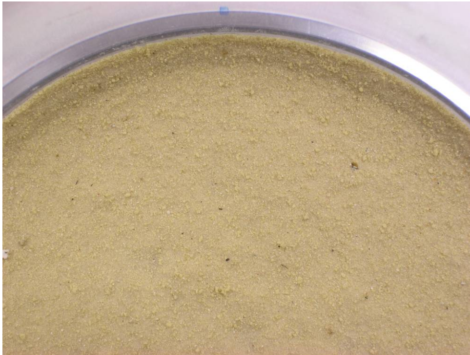
Figure J.13.4. Close-Up of 051128_NC_2776_L2 Debris Bed in Test Section After Retrieval, Top View.
