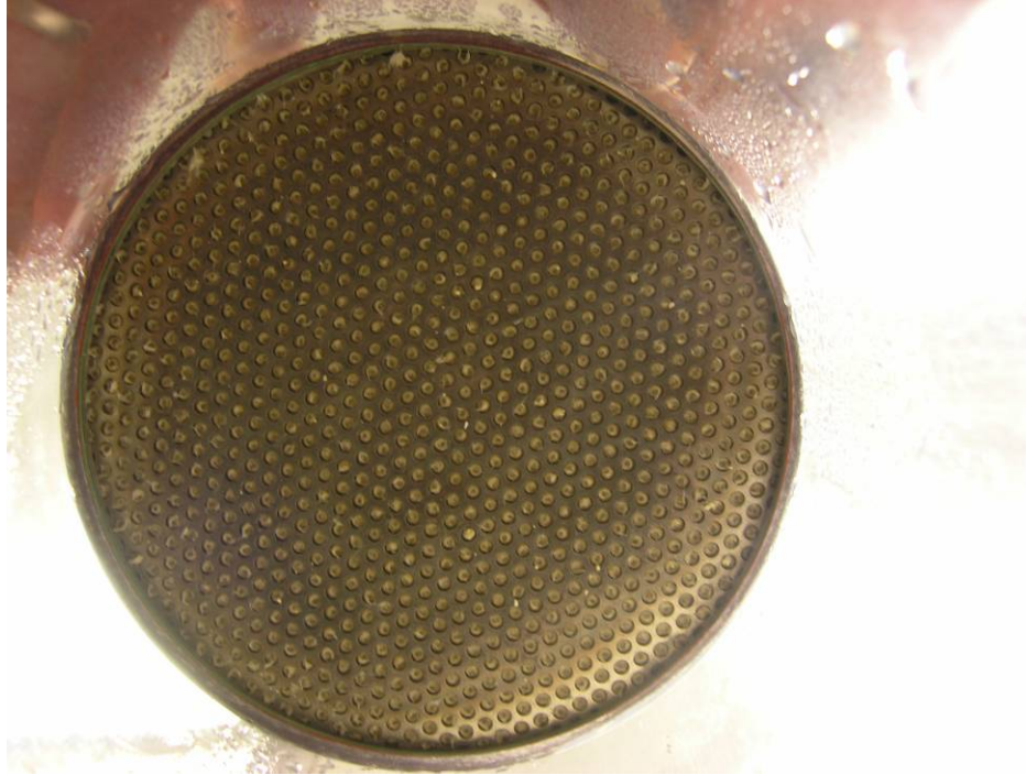
Figure J.9.4. 060331_NC_2024_LP1 Debris Bed in Test Section After Retrieval, Bottom View
