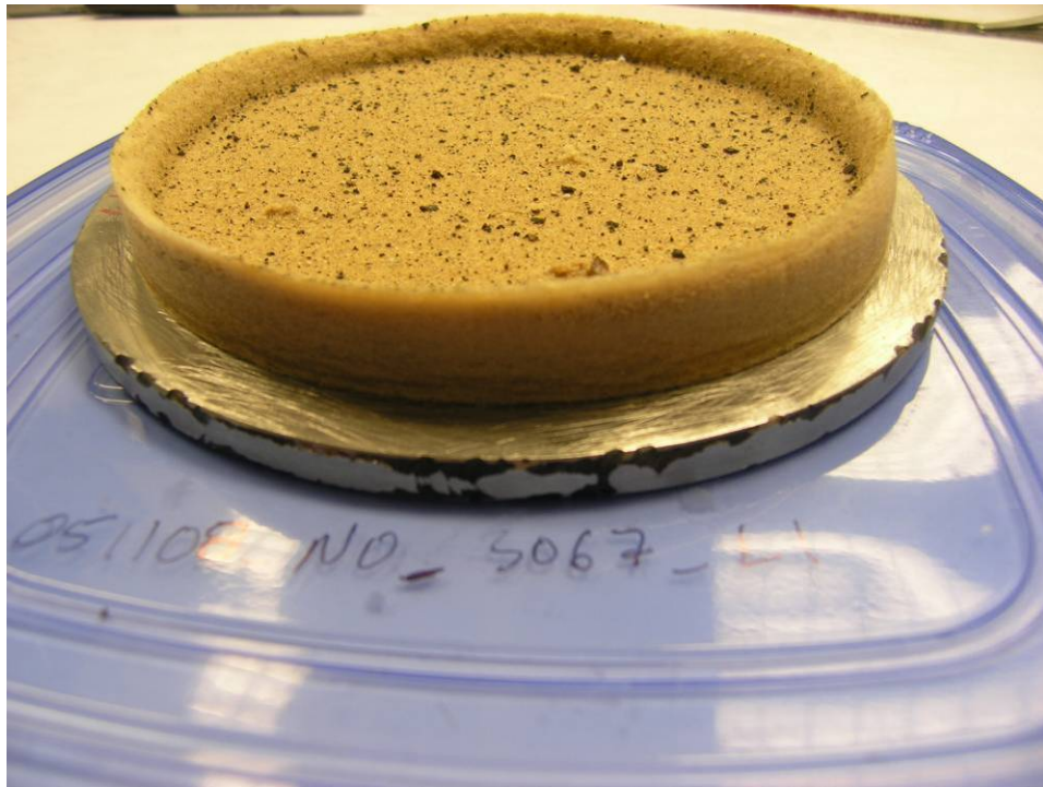
Figure H.4.6. 051108_NO_3067_L1 Debris Bed After Retrieval from Test Section
