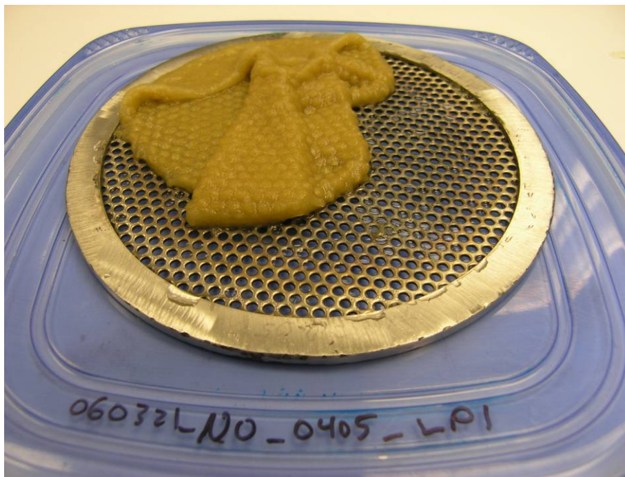
Figure H.1.3. 060321_NO_0405_LP1 Debris Bed After Retrieval. The disturbance consisted of the entire debris bed floating up under severely reduced flow conditions, flipping over and folding up, and then re-depositing on the plate once flow was increased. The debris bed was visually observed to remain essentially intact.
