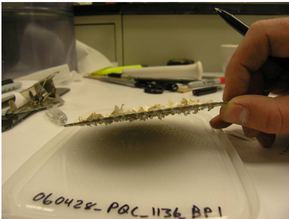
Figure J.2.3. Edge View of Retrieved Paint Chip Debris Bed from Test 060428_PQC_1136_BP1
