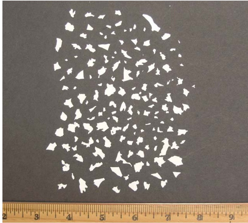
Figure O.1.2. Size Characterization Photo for ALK-Chips Debris. Total mass of particulate in photo was 0.17 g.
