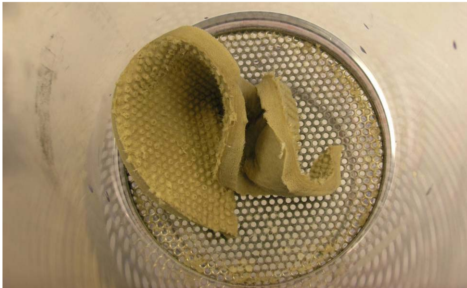
Figure J.10.4. 060404_NC_2698_LP1 Debris Bed in Test Section After Retrieval, Top View. The disturbance resulted from unequal cover-gas pressure around the debris bed post-draining. After test BM-3, a vent was added below the debris bed to allow the test loop to be drained and gas pressure equalized without rupture (Figure J.10.3), even with the relative impermeability of the debris bed. The impermeability resulted in water being held above and an air void below. While removing the water, a portion of the test loop below the debris bed was isolated while under pressure. Subsequent opening of this portion of the test loop before removing the debris bed resulted in the rupture. Test procedures will be modified to prevent reoccurrence.
