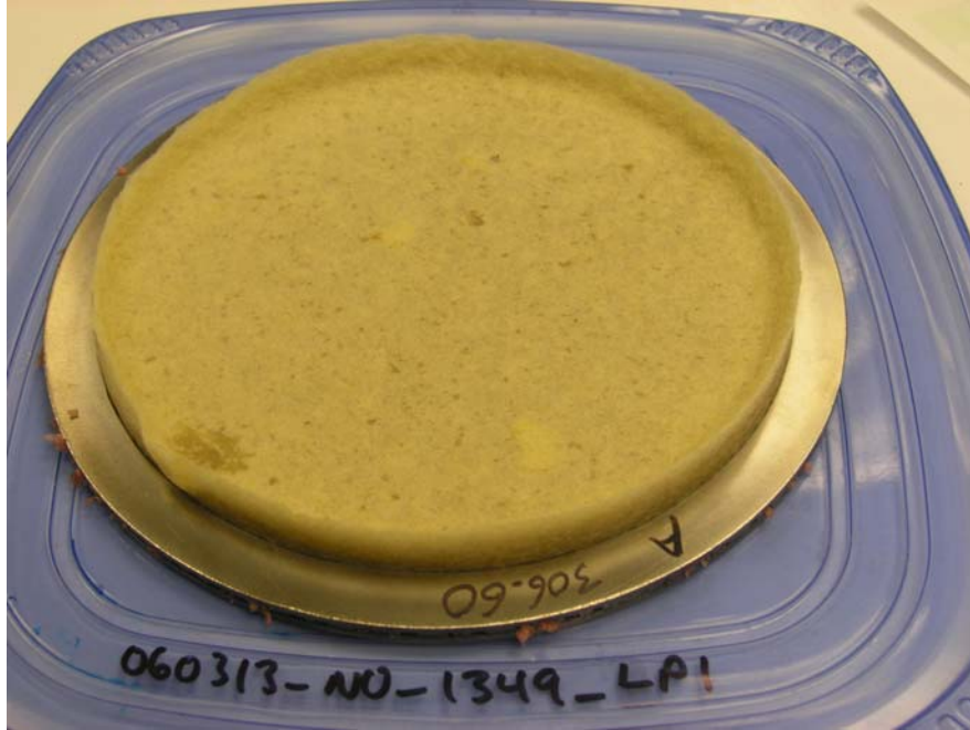
Figure H.2.4. 060313_NO_1349_LP1 Debris Bed After Retrieval from Test Section
