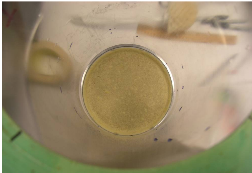
Figure J.8.3. 060323_NC_1619_LP1 Debris Bed in Test Section After Retrieval, Top View
