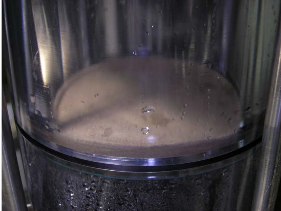
Figure H.5.3. 060125_NO_3067_L1 Debris Bed in Large Scale Loop After Draining
