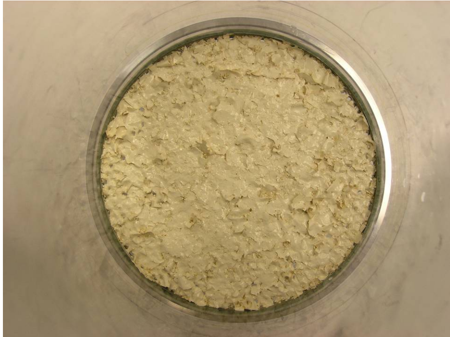
Figure K.1.5. 060501_PQC_2609_LP1, LP2 Debris Bed in Test Section After Retrieval, Top View
