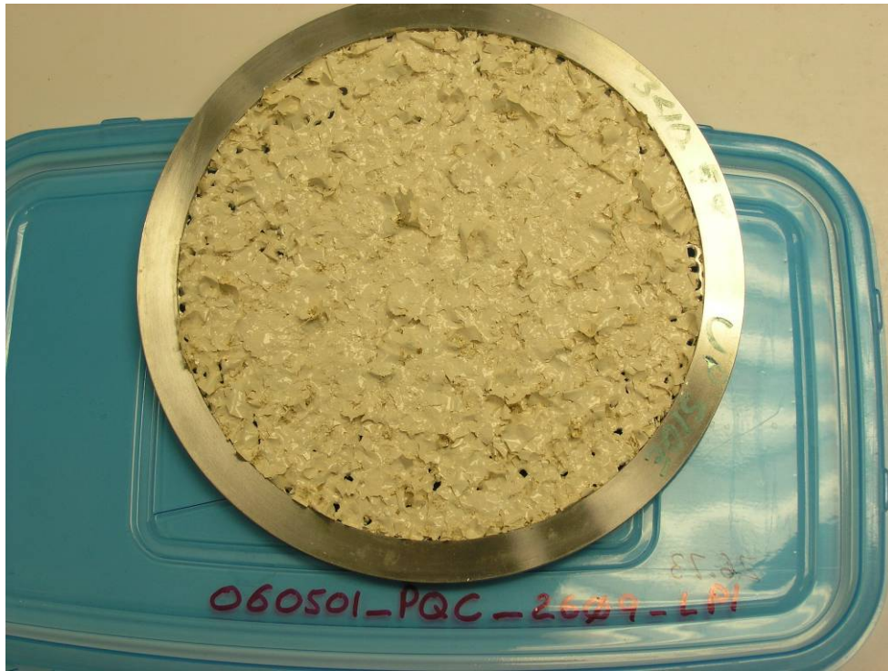
Figure K.1.7. 060501_PQC_2609_LP1, LP2 Debris Bed After Retrieval from Test Section, Top View
