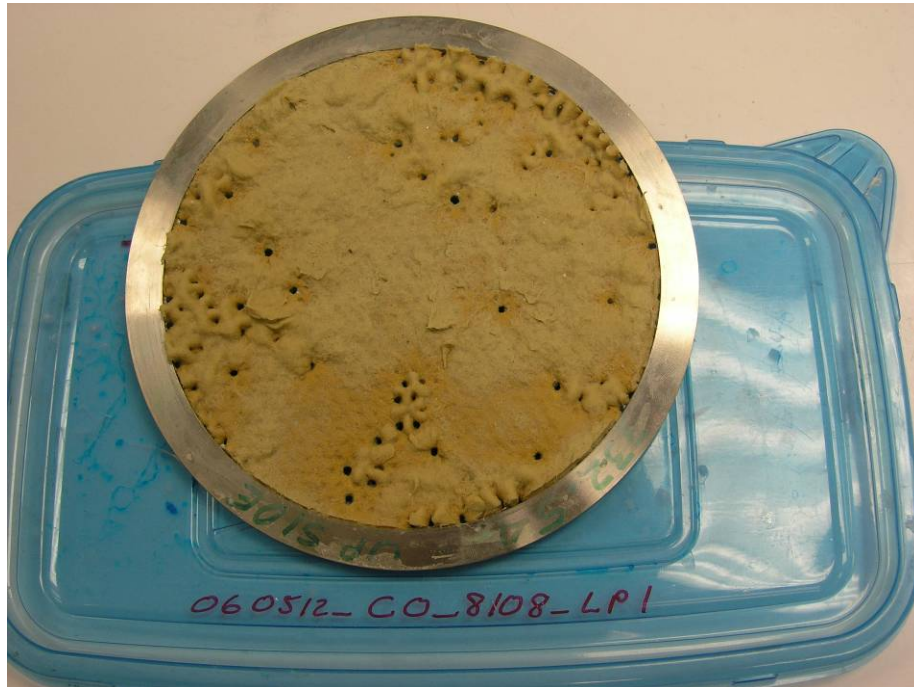
Figure I.2.8. 060512_CO_8108_LP1, LP2, and LP3 Debris Bed After Retrieval from Test Section
