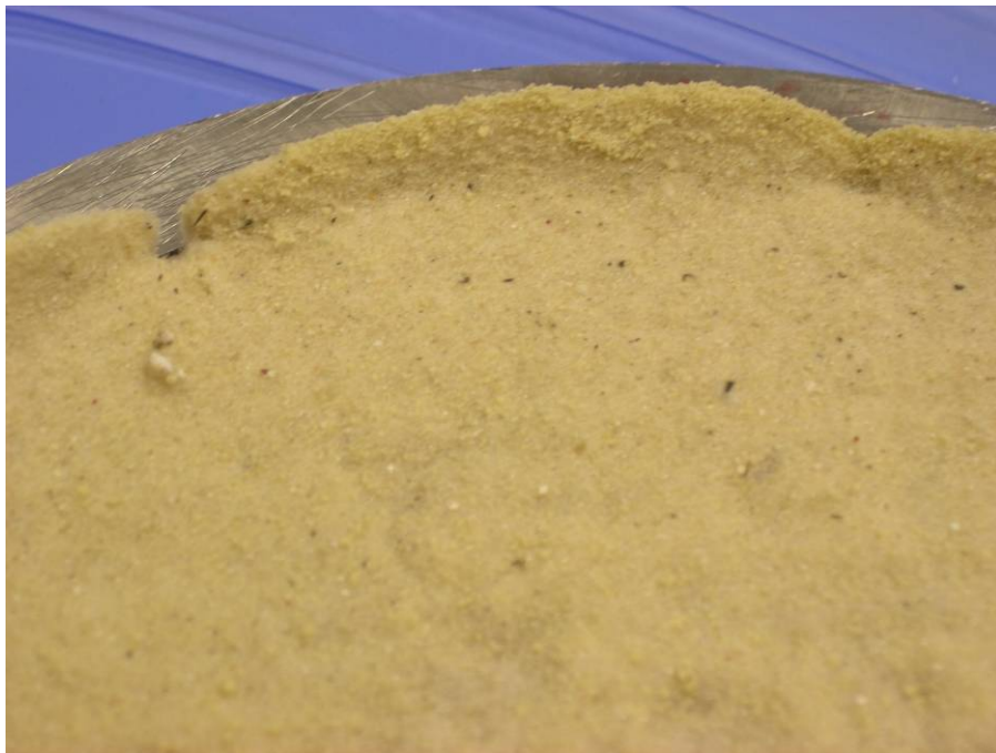
Figure J.11.8. Close-up of 051123_NC_2181_L1 Debris Bed After Retrieval from Test Section. Screen pattern is observable on debris bed surface; flow channels are observable on debris bed edge.
