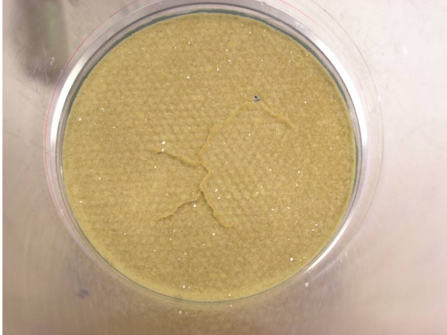
Figure J.4.2. Debris Bed in Test Section After Retrieval, Top View; Disturbed Post-Test
