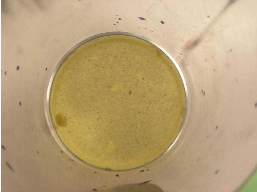
Figure H.2.2. 060313_NO_1349_LP1 Debris Bed in Test Section After Retrieval, Top View
