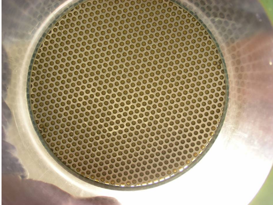
Figure H.3.5. 060425_NO_2703_LP1, LP2, LP3 Debris Bed in Test Section After Retrieval, Bottom View
