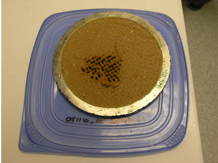
Figure J.3.5. Ruptured 051110_NC_0595_L1 Debris Bed After Retrieval from Test Section; Rupture Caused Post-Test
