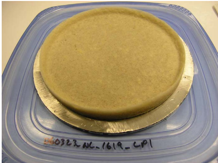
Figure J.8.5. 060323_NC_1619_LP1 Debris Bed After Retrieval from Test Section
