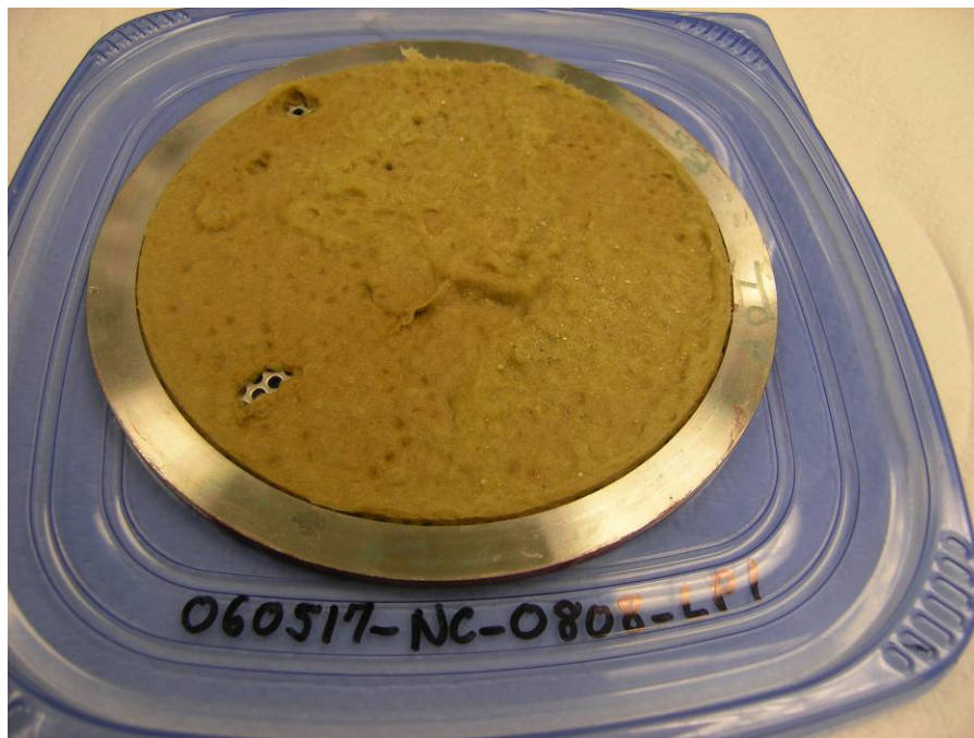
Figure J.6.6. 060517_NC_0808_LP1, LP2 Debris Bed After Retrieval from Test Section. Debris bed disturbed during retrieval (see Figure J.6.3 caption).
