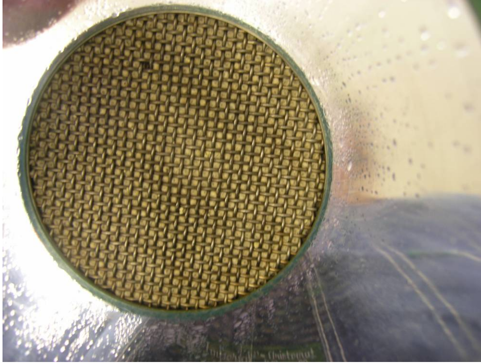
Figure J.13.5. 051128_NC_2776_L2 Debris Bed in Test Section After Retrieval, Bottom View
