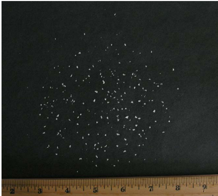
Figure O.1.1. Size Characterization Photo for ALK-Processed Debris. Total mass of particulate in photo was 0.01 g.
