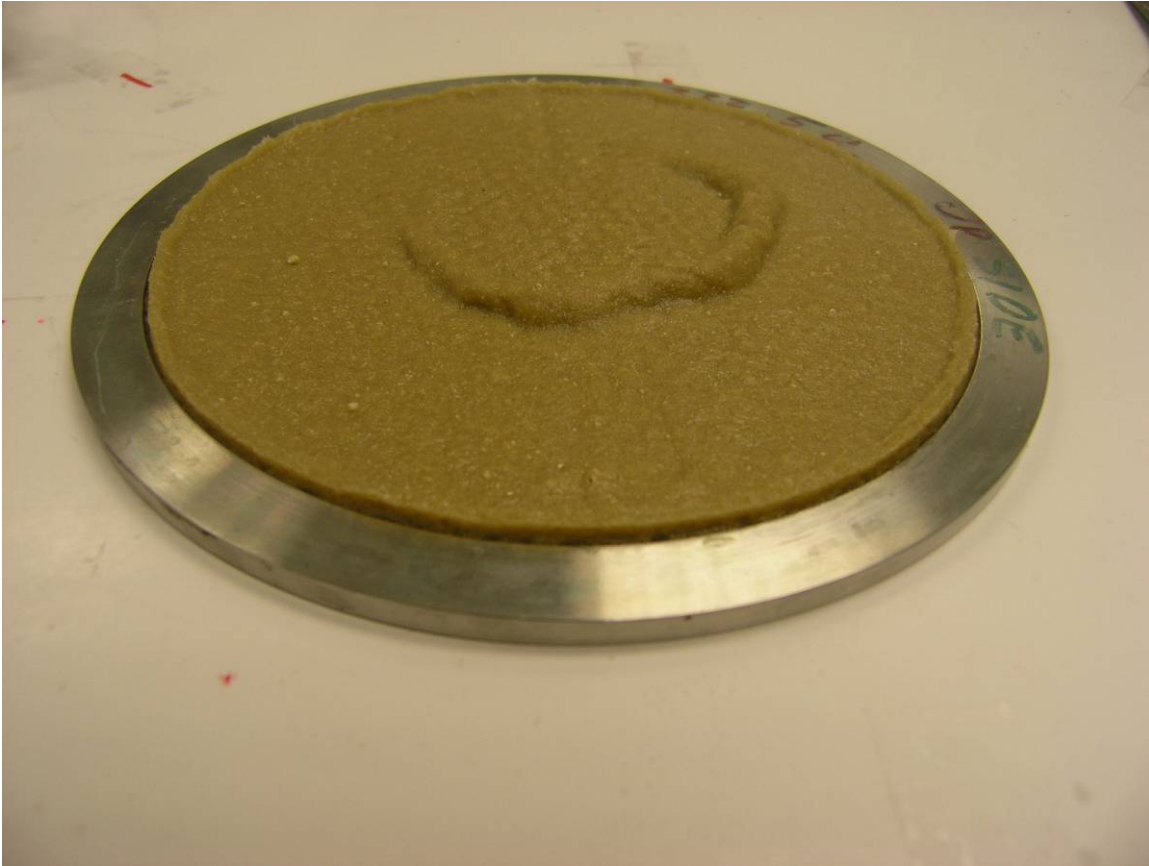
Figure J.15.5. Debris Bed After Retrieval from Test Section. Disturbed post-test.
