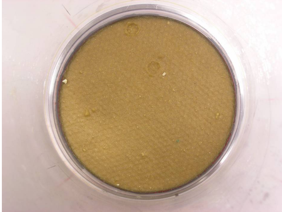
Figure J.16.3. Debris Bed in Test Section After Retrieval, Top View. Disturbed post-test.
