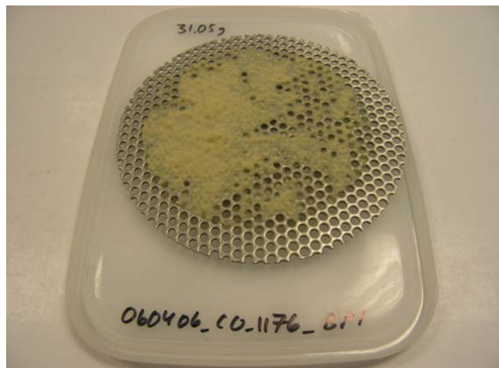
Figure I.1.1. 060406_CO_1176_BP1 Debris Bed Post-Retrieval
