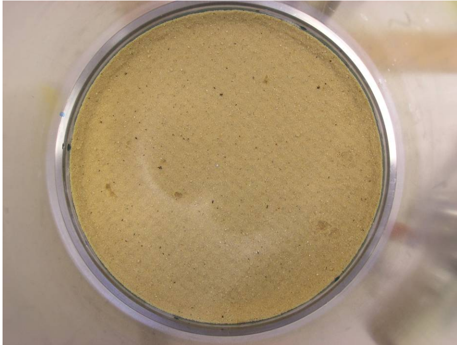
Figure J.7.4. 051121_NC_1586_L1 Debris Bed in Test Section After Retrieval, Top View. Screen pattern is observable on debris bed surface; dark pock-marks are from post-retrieval water drips.
