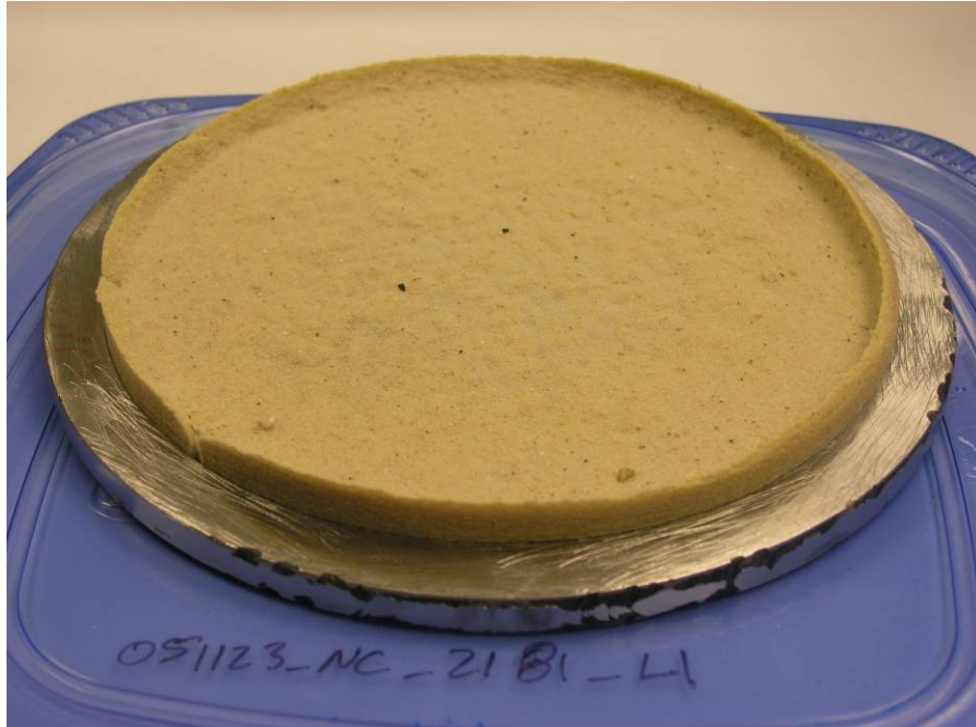
Figure J.11.7. 051123_NC_2181_L1 Debris Bed After Retrieval from Test Section. Screen pattern is observable on debris bed surface; flow channels are observable on left side of debris bed.
