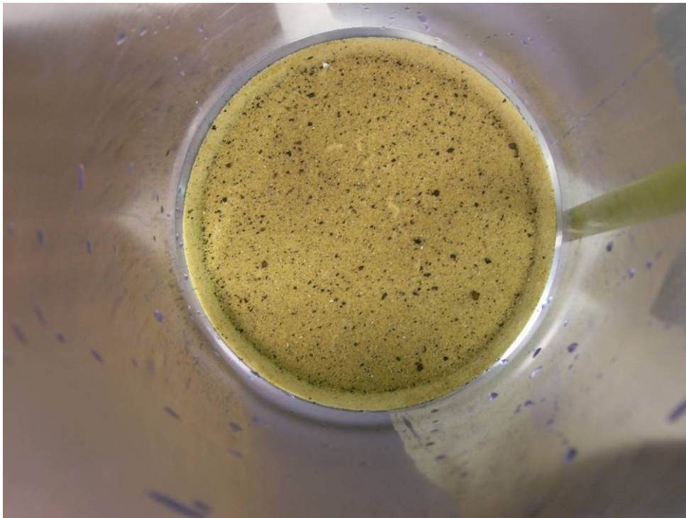
Figure H.4.4. 051108_NO_3067_L1 Debris Bed in Test Section After Retrieval, Top View
