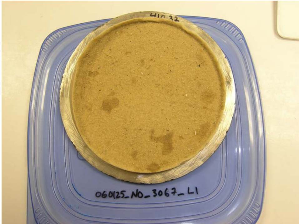
Figure H.5.5. 060125_NO_3067_L1 Debris Bed After Retrieval from Test Section
