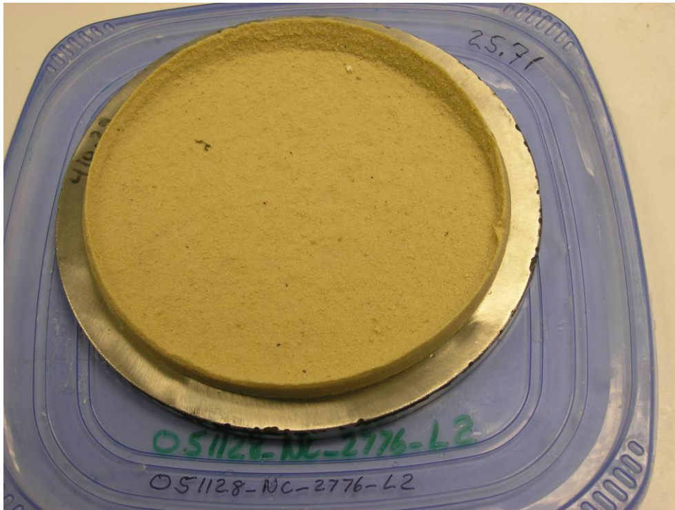
Figure J.13.6. 051128_NC_2776_L2 Debris Bed After Retrieval from Test Section. Indentation on Debris Bed Rim at 3:15 Orientation Due to Post-Retrieval Handling.
