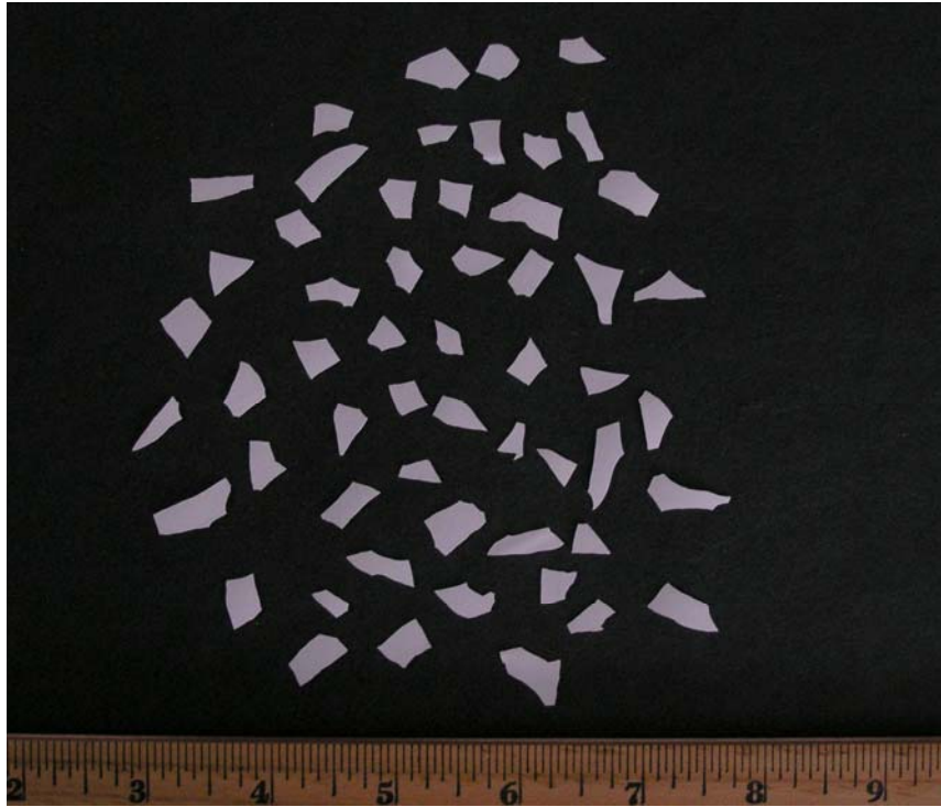
Figure O.1.4. Size Characterization Photo for ZE-Chips Debris. Total mass of particulate in photo was 1.0 g.
