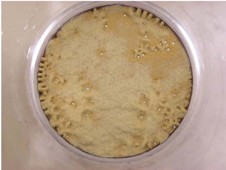
Figure I.2.6. 060512_CO_8108_LP1, LP2, and LP3 Debris Bed in Test Section After Retrieval, Top View
