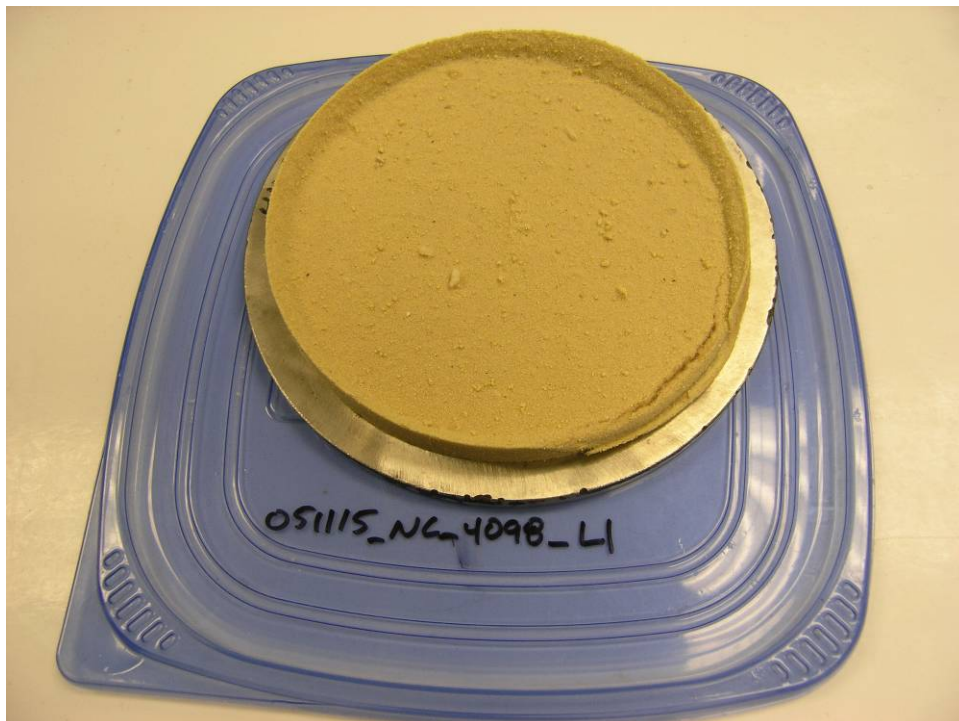
Figure J.14.6. 051115_NC_4098_L1 Debris Bed After Retrieval from Test Section. Collapsed rim was caused following test section retrieval from test loop.
