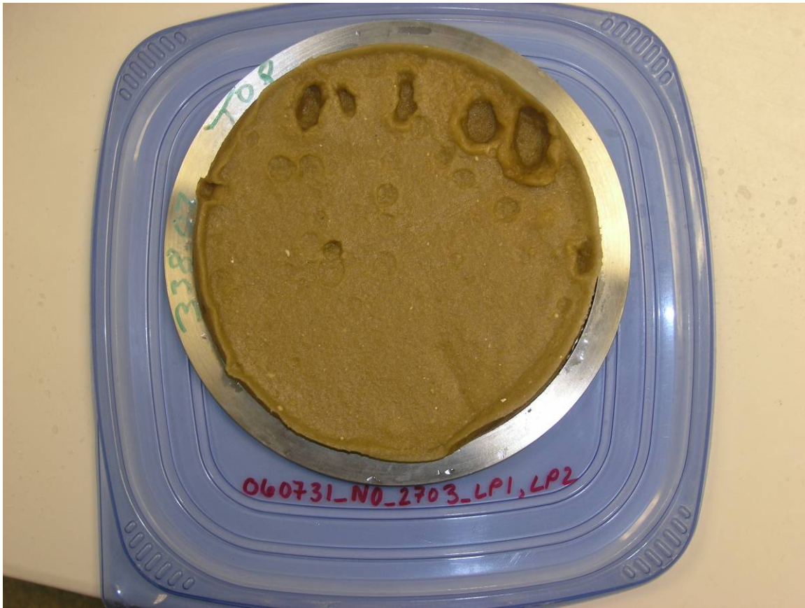
Figure H.6.5. Debris Bed After Retrieval from Test Section, Disturbed Post-Test
