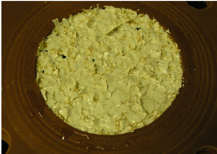
Figure J.2.1. Paint Chip Debris Bed from Test 060428_PQC_1136_BP1 before Removing Debris Bed from Test Section. The target debris loading was 1.4 kg/m 2 with a 1 to 1 ratio of 1/4-inch-square to processed material.
