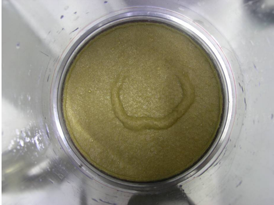
Figure J.15.3. Debris Bed in Test Section After Retrieval, Top View. Disturbed post-test.
