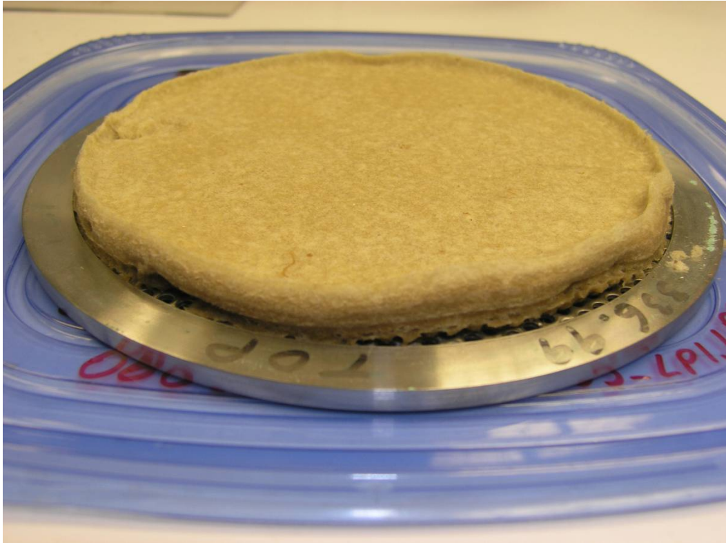
Figure H.7.5. Debris Bed After Retrieval from Test Section. Disturbed post-test.
