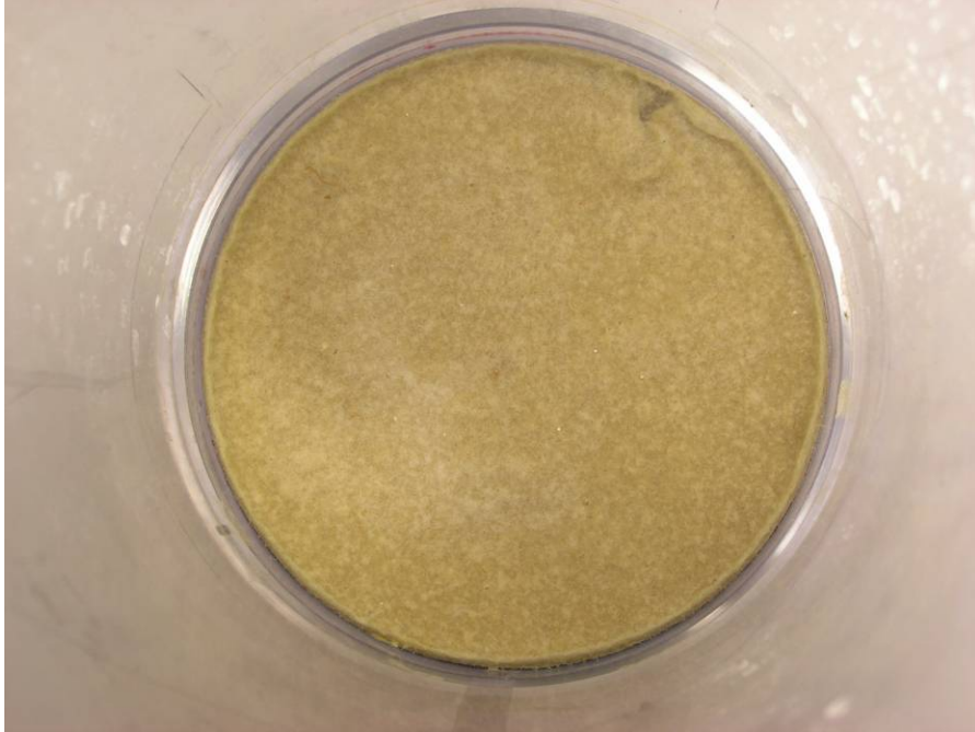
Figure H.7.3. Debris Bed in Test Section After Retrieval, Top View. Disturbed post-test.
