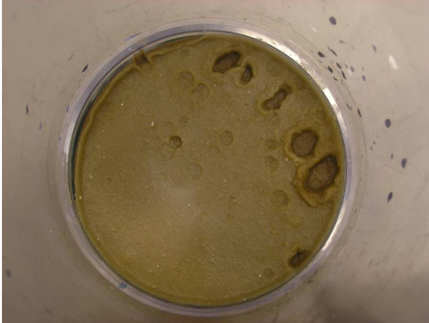
Figure H.6.3. Debris Bed in Test Section After Retrieval, Top View. Disturbed post-test.
