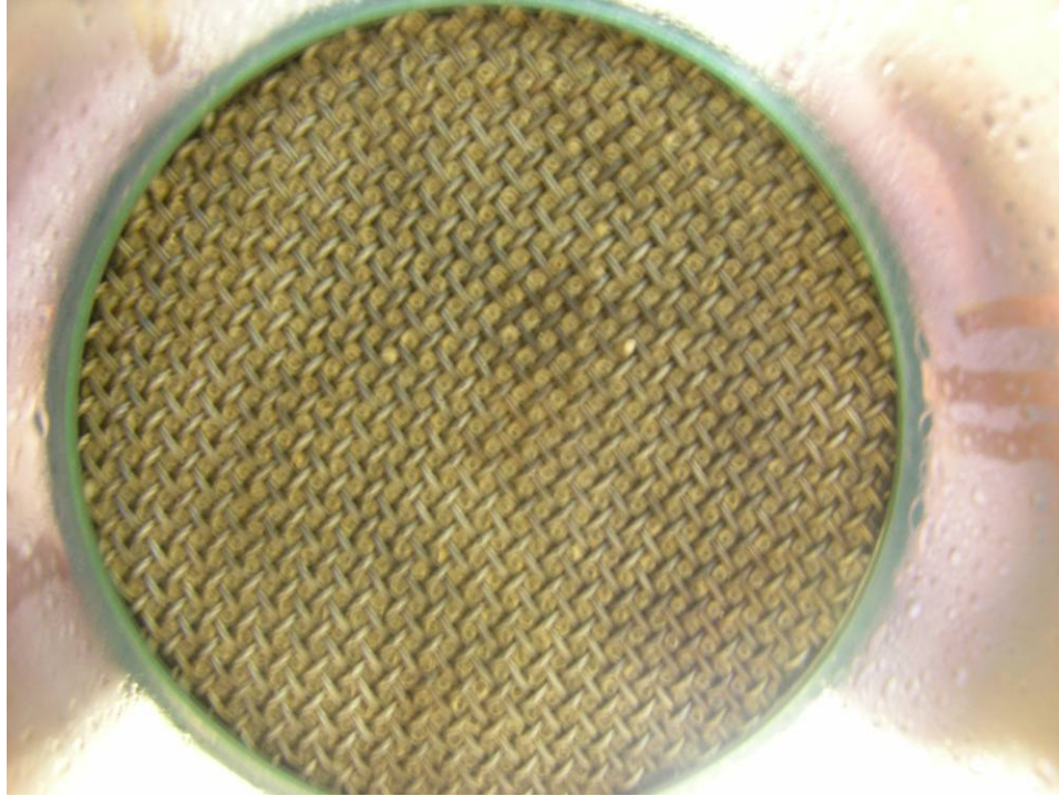
Figure H.4.5. 051108_NO_3067_L1 Debris Bed in Test Section After Retrieval, Bottom View
