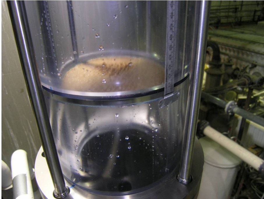
Figure J.3.3. Ruptured 051110_NC_0595_L1 Debris Bed After Draining; Rupture Caused Post-Test
