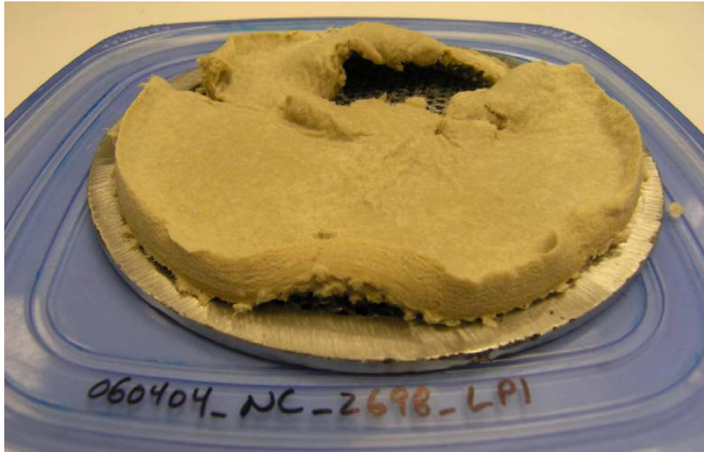
Figure J.10.5. 060404_NC_2698_LP1 Debris Bed After Retrieval from Test Section (laid flat after rupture of Figure J.29)
