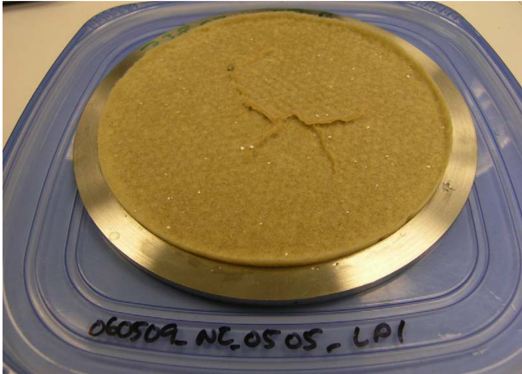
Figure J.4.4. Debris Bed After Retrieval from Test Section; Disturbed Post-Test
