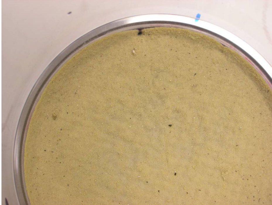
Figure J.11.5. Close-Up of 051123_NC_2181_L1 Debris Bed in Test Section After Retrieval, Top View. Screen pattern is observable on debris bed surface; flow channels are observable at 11:45 and 1:30 orientations.
