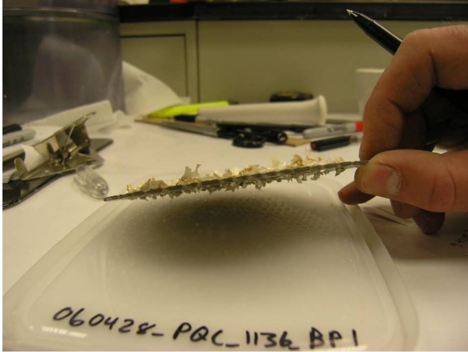
Figure K.1.13. 060428_PQC_1136_BP1 Debris Bed Post-Retrieval, Edge View (note penetration of ALK debris into perforations of plate)
