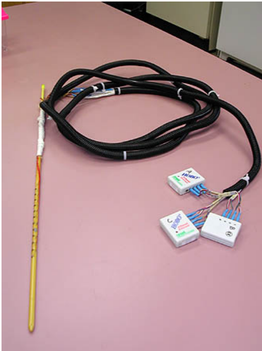
Photo 7: A fiberglass probe was impregnated with a row of thermistors attached to dataloggers to continuously record maggot mass temperatures through time and space.
