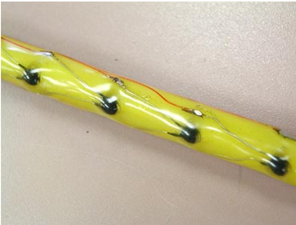
Photo 8: A close-up view of some of the temperature probe thermistors. They were spaced 1.5cm apart.
