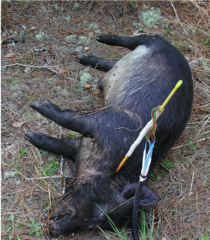
Photo 9: The temperature probe is seen here inserted into a pig carcass. Because of the wound that is made, the probe site becomes a focus of maggot colonization.
