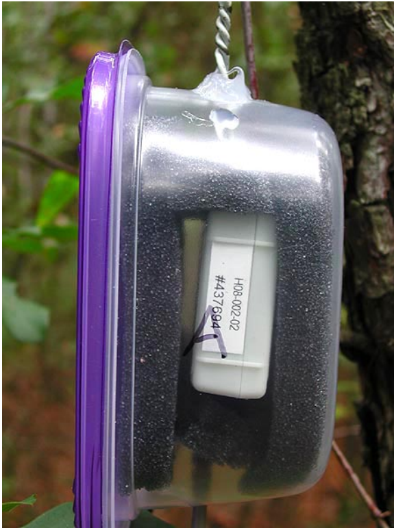
Photo 1: A datalogger protected in a plastic container was suspended near each pig carcass to record ambient temperature for the duration of each trial. The temperature probe extends from the box to hang in the open air.
