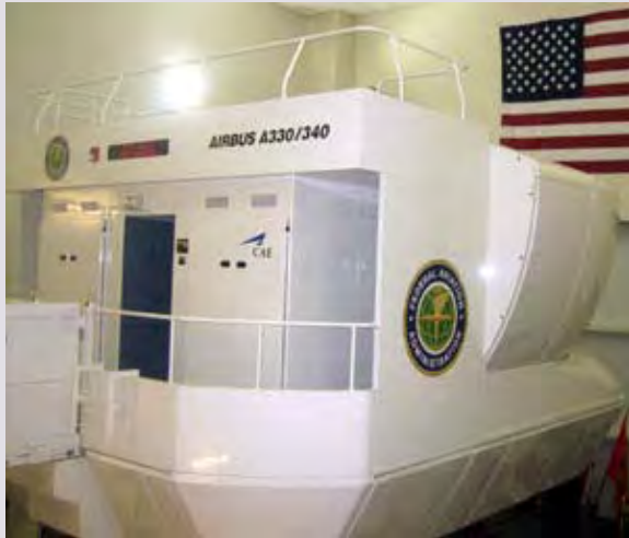
The FAA's Airbus 330/340 simulator equipped with NextGen technology allows new safety and efficiency concepts to be researched and tested.
