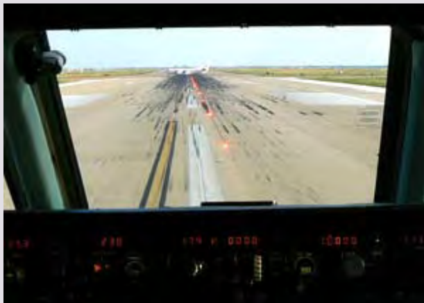
RWSL systems are fully automatic and designed to reduce the number and severity of runway incursions.
