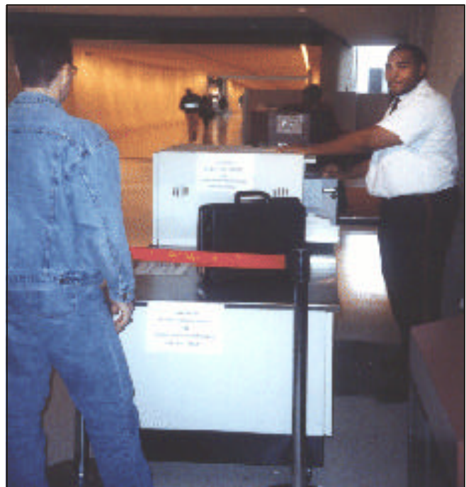
Bulk explosive detection devices for screening checked bags are being deployed at the Nation's busiest airports.
