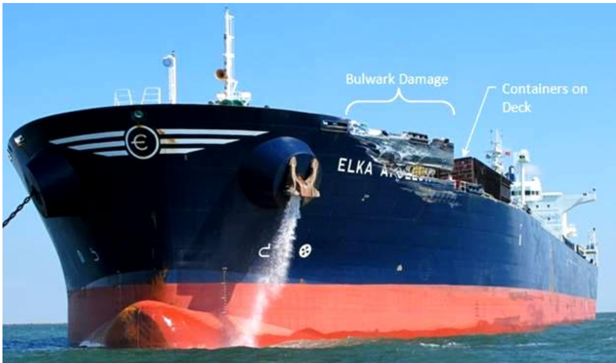
Figure 5. Damage to Elka Apollon port bow and partial view of containers that fell to its deck from the MSC Nederland .
