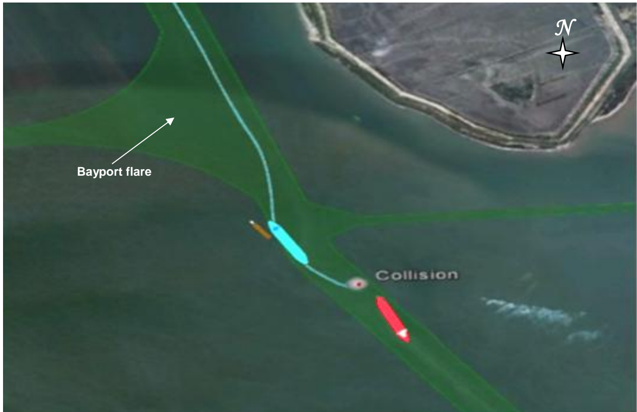
Figure 11. Trackline of the Elka Apollon (blue) and positions of the MSC Nederland (red) and the Mr. Earl (brown) at 0904:29, about 1 minute before the accident.
