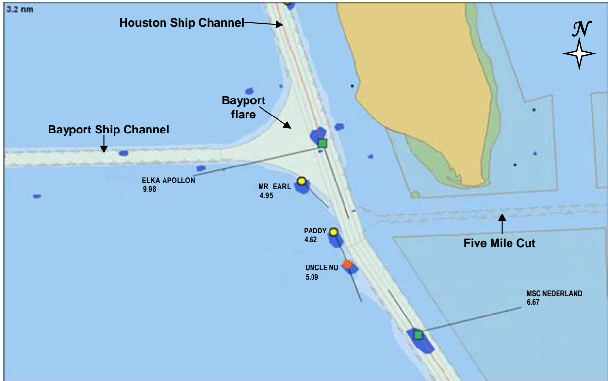
Figure 10. Portion of VTS AIS display at 0902 on October 29, 2011, showing the Elka Apollon outbound and the MSC Nederland inbound (green squares near center and bottom right of screen, respectively) as they approach each other near the slight bend in the Houston Ship Channel and Five Mile Cut. The Mr. Earl is indicated by the uppermost yellow circle. The two other tows in the barge lane are labeled Paddy (yellow circle) and Uncle Nu (orange circle). Below the vessel name is its speed in knots. The dark blue areas near the vessel locations are radar images. (Original AIS vessel labels have been simplified for readability.)
