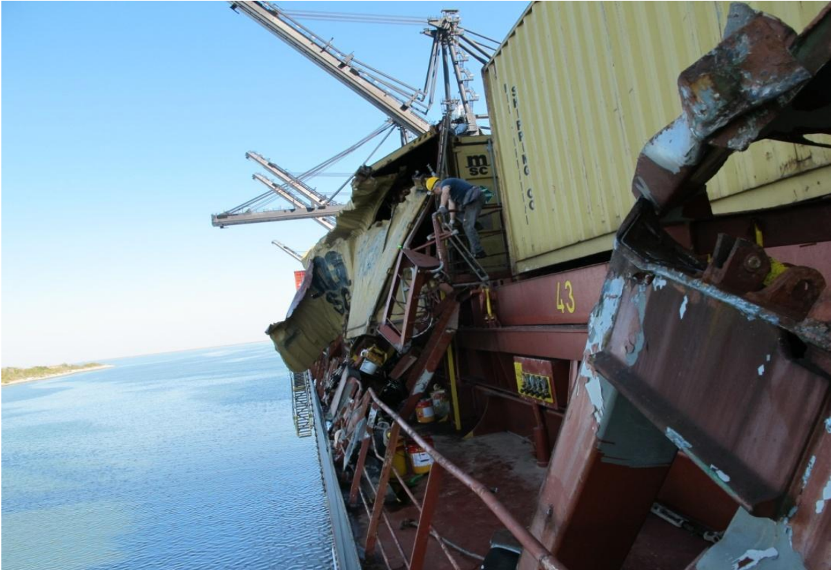
Figure 6. MSC Nederland damage, looking forward from superstructure at main deck.
