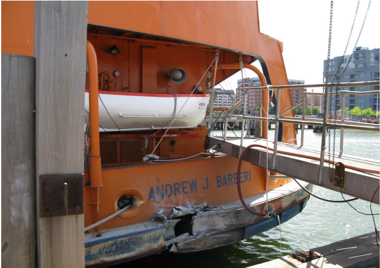
Figure 8. Damage to the vessel's starboard side (Staten Island-end).
