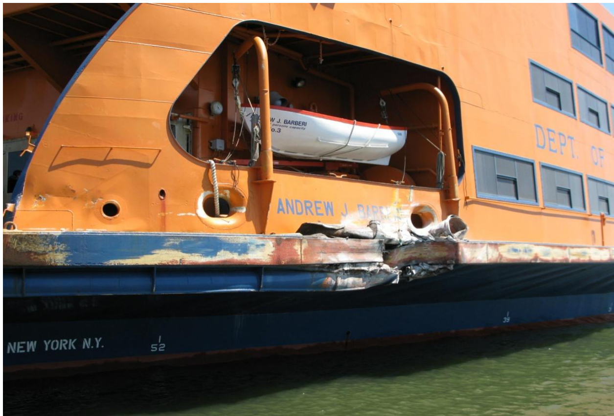
Figure 7. Damage to the vessel's port side (Staten Island-end).
