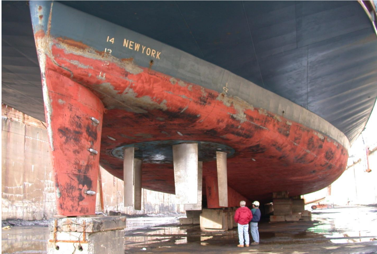
Figure 9. One of the two cycloidal propellers on the Andrew J. Barberi .
