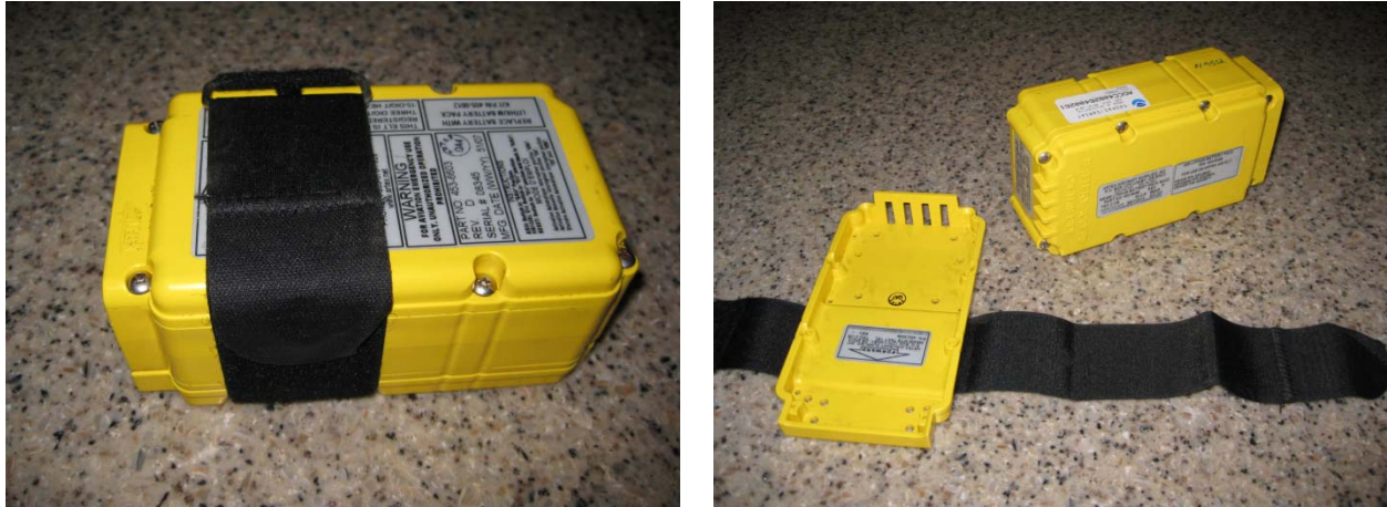
Figure 13. Two views of the accident airplane's emergency locator transmitter's (ELT) retention system.
