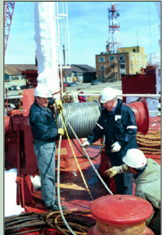
Left to right – Terrance Jordan, SLSDC, and Captain Lajarrige, SLSMC, measure one of the forward mooring wire eyes to assure that they are the proper length. Kneeling is the Chief Officer of the vessel.
