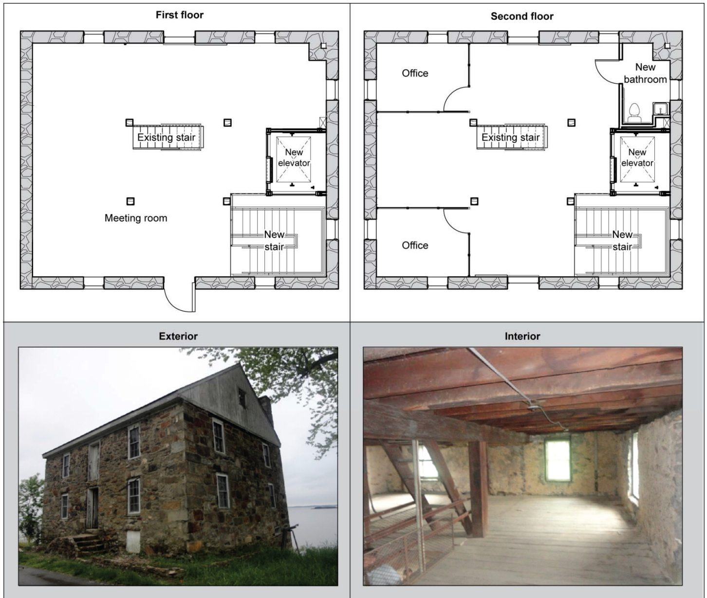
Figure 4: VA—Proposed Design for VA’s Old Grist Mill at Perry Point, Maryland, Including New Stair, Elevator, and Bathroom
