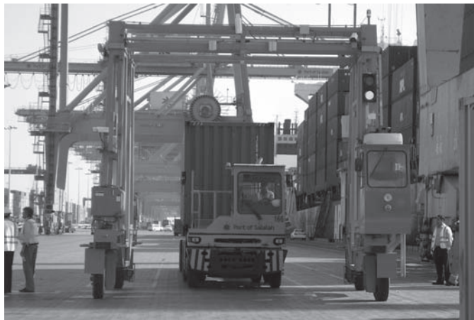
Radiation detection equipment known as Mobile Radiation Detection Identification System (MRDIS), Port of Salalah, Oman
