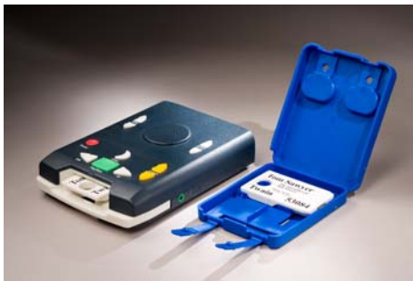
Figure 2: Advanced (top) and standard DTBM with flash cartridge.
