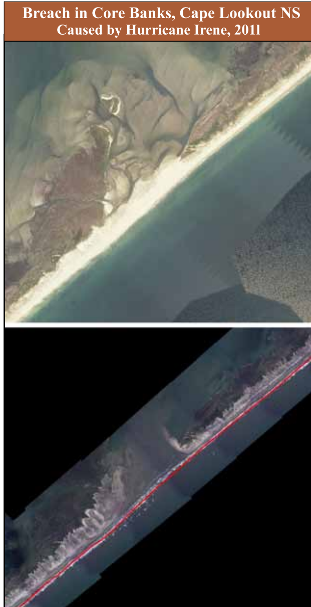
Figure 7. Photographs of Core Banks, Cape Lookout NS, from June 12, 2010 (upper) and August 28, 2011, one day after landfall of Hurricane Irene. The red line in the lower photo is the location of the oceanfront shore on June 12, 2010. A breach has been cut through the barrier island. Source of photographs: NOAA. 75
