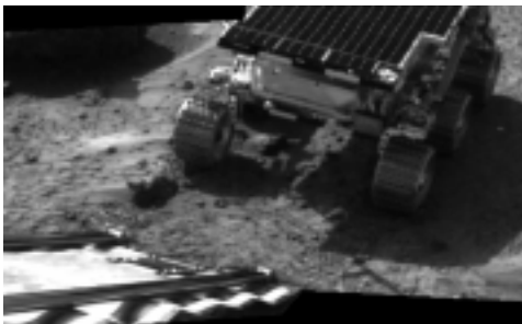
Top: Sojourner's descent on the right ramp was successful. Soil beneath the rover is the first target of the alpha proton X-ray spectrometer (APXS). Middle: Sojourner appears in one of the first images taken by the Imager for Mars Pathfinder (IMP) on Sol 3. Bottom: APXS is shown here placed against soil at the base of "Yogi."
