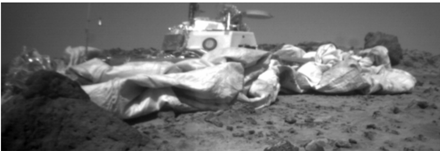
The "Mini Matterhorn" is shown at lower left in this image of the lander with its deflated airbags in the foreground.
