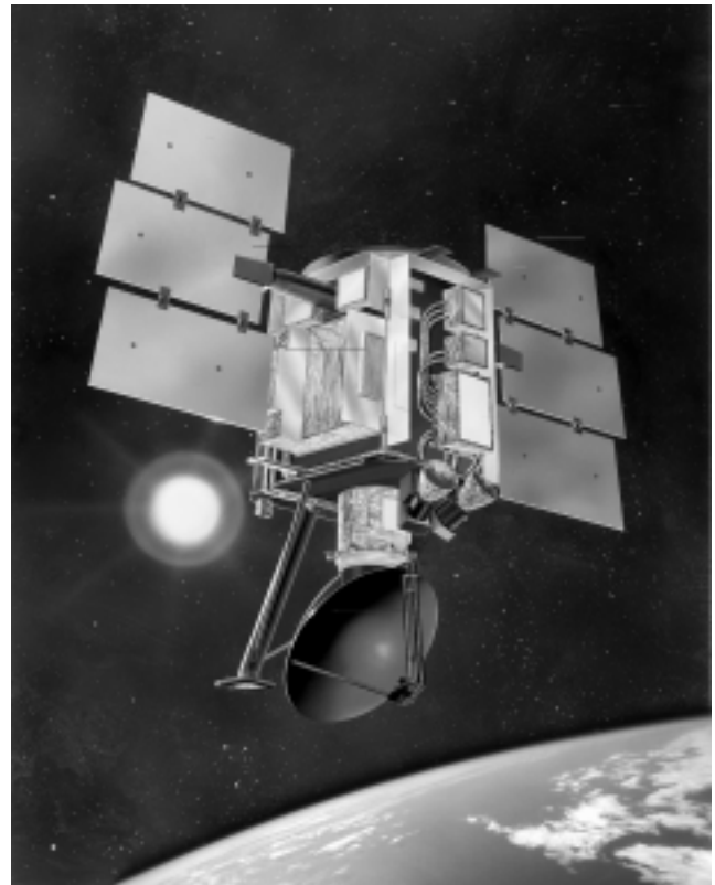
The QuikSCAT satellite carries the SeaWinds instrument — a special microwave radar that measures wind speed near the surface of Earth’s oceans. SeaWinds will continue the collection of ocean wind data begun by NSCAT.
