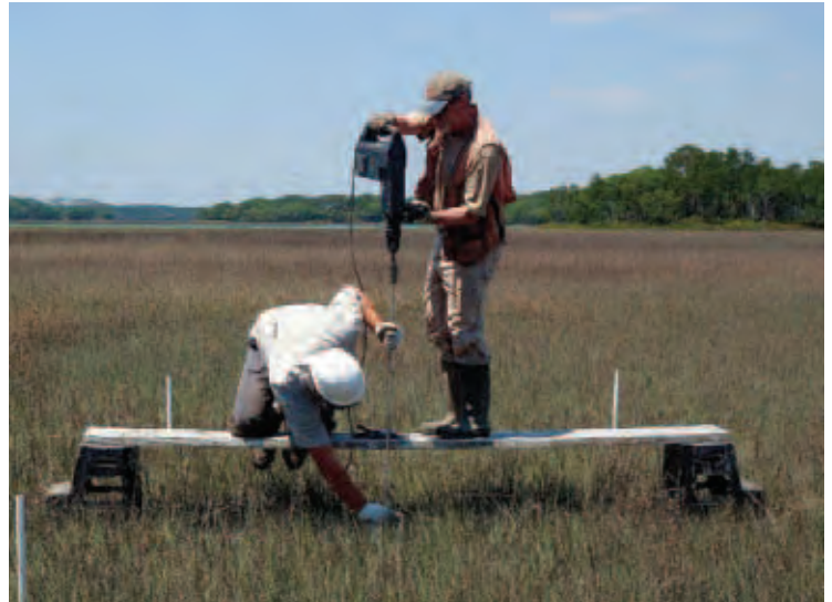
Scientists Dave O'Loughlin and Jeremy Schmid of Atkins Global, an engineering consulting firm, install a rod surface elevation table (RSET) benchmark at Pinckney Island National Wildlife Refuge, SC. The Southeast Region Inventory and Monitoring (I&M) Network is monitoring marsh elevation at 18 coastal refuges. (Nicole Rankin/USFWS)
