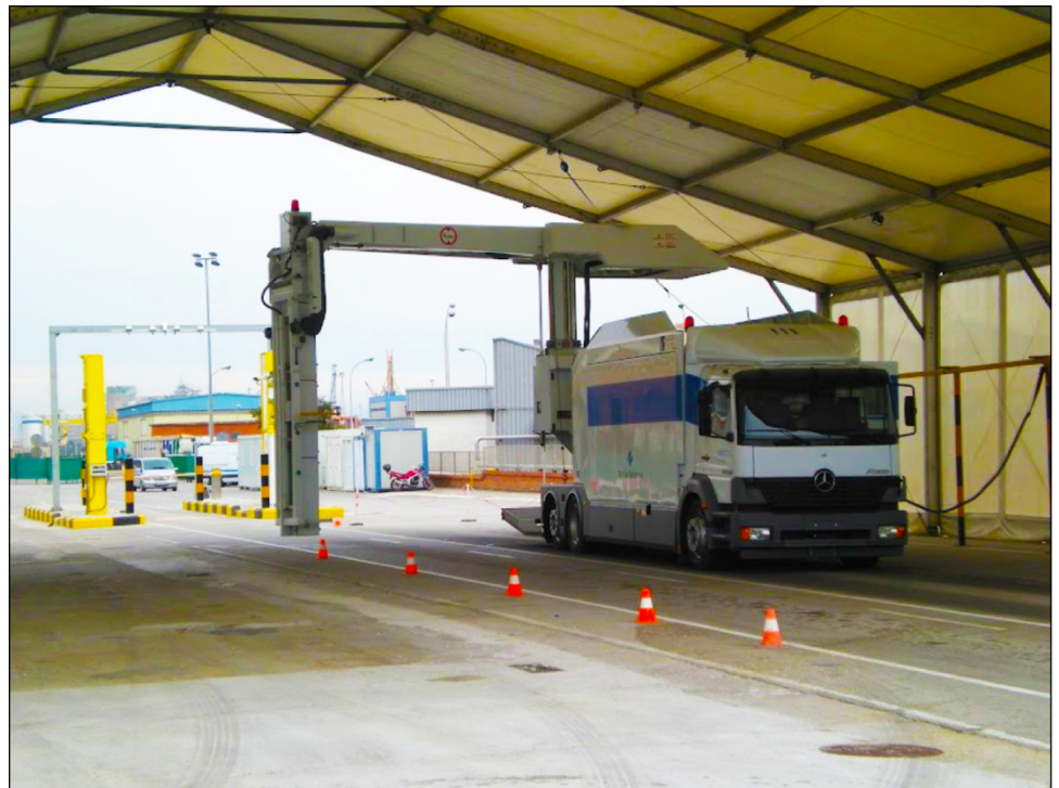
Figure 6: CSI Nonintrusive Imaging System Next to the Megaports Initiative's Radiation Detection Scanning Equipment
