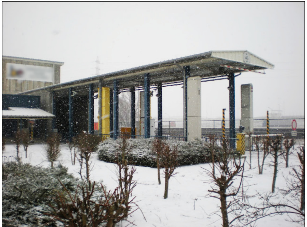
Figure 5: A Spectroscopic Portal Monitor Used for Secondary Radiation Detection Scanning
