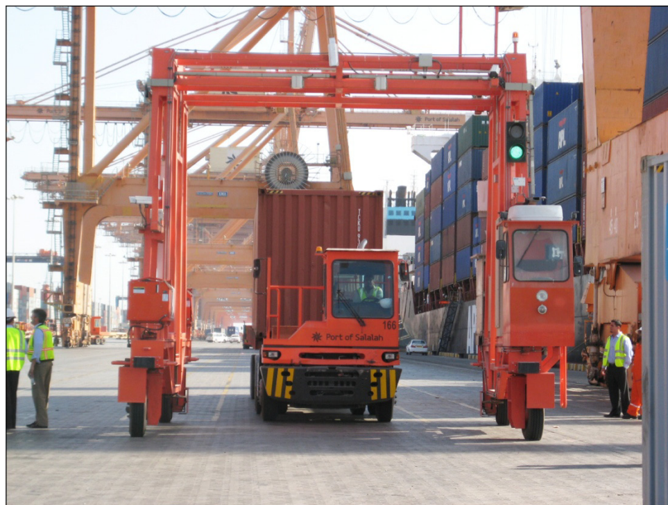
Figure 3: Truck Driving through a Mobile Radiation Detection and Identification System
