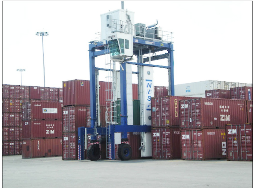
Figure 4: Radiation Detection Straddle Carrier Scanning Shipping Containers
