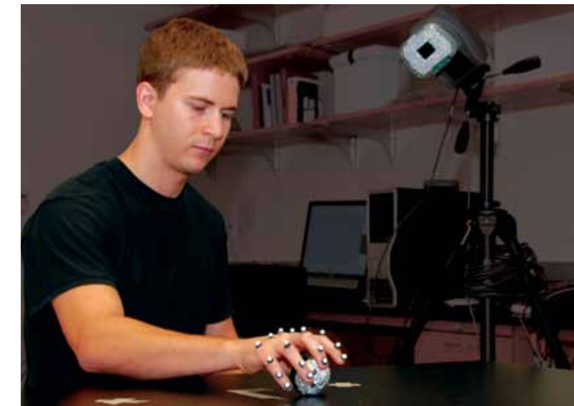
Sam Durham, PMI Research Engineer, demonstrates sensors used to record and measure hand movements.
