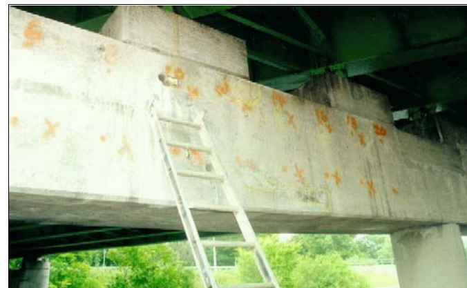
Figure 2-2. Views of test sections on: (a) south pier (control), (b) middle pier (Cortec 2000), and (c) north pier (DCI).
