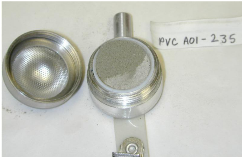
Figure 1. Loose particulate inside a shielded BAS active sample. The external shield that would go over the protective screen is not shown.
