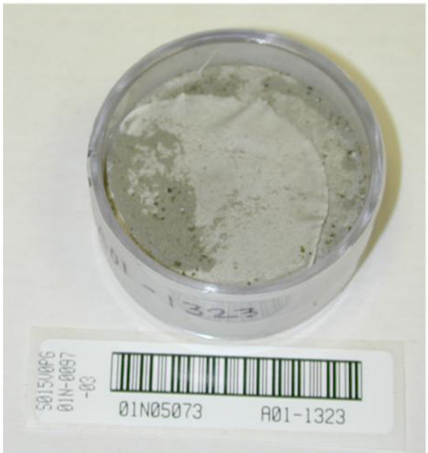
Figure 2. Loose particulate and a damaged filter from a 37-mm filter cassette active sample.
