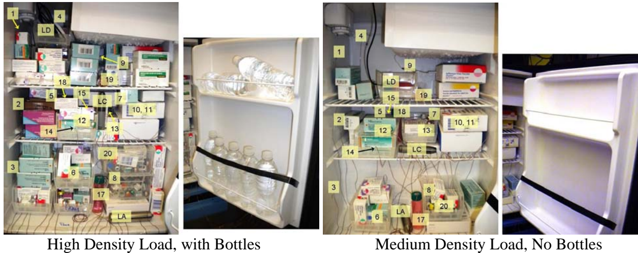
Fig. 21. Refrigerator loading at different densities and with and without water bottles.
