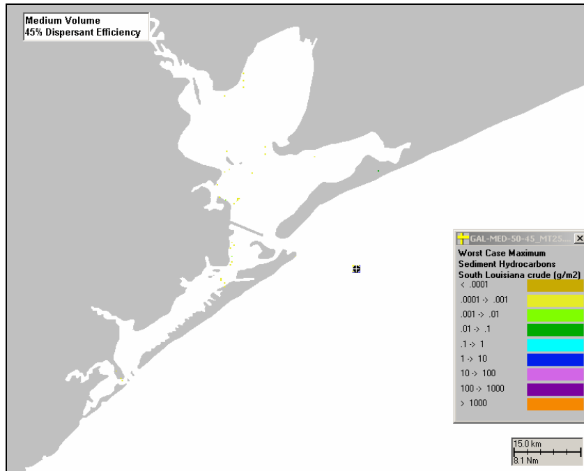
Figure C-II.1.2.5-2 Sediment exposure to total hydrocarbons ( \text{g}/\text{m}^2 ) under worst-case environmental conditions for each location (i.e., maximum possible exposure). Scenario: Medium Volume, 45% Dispersant Efficiency.
