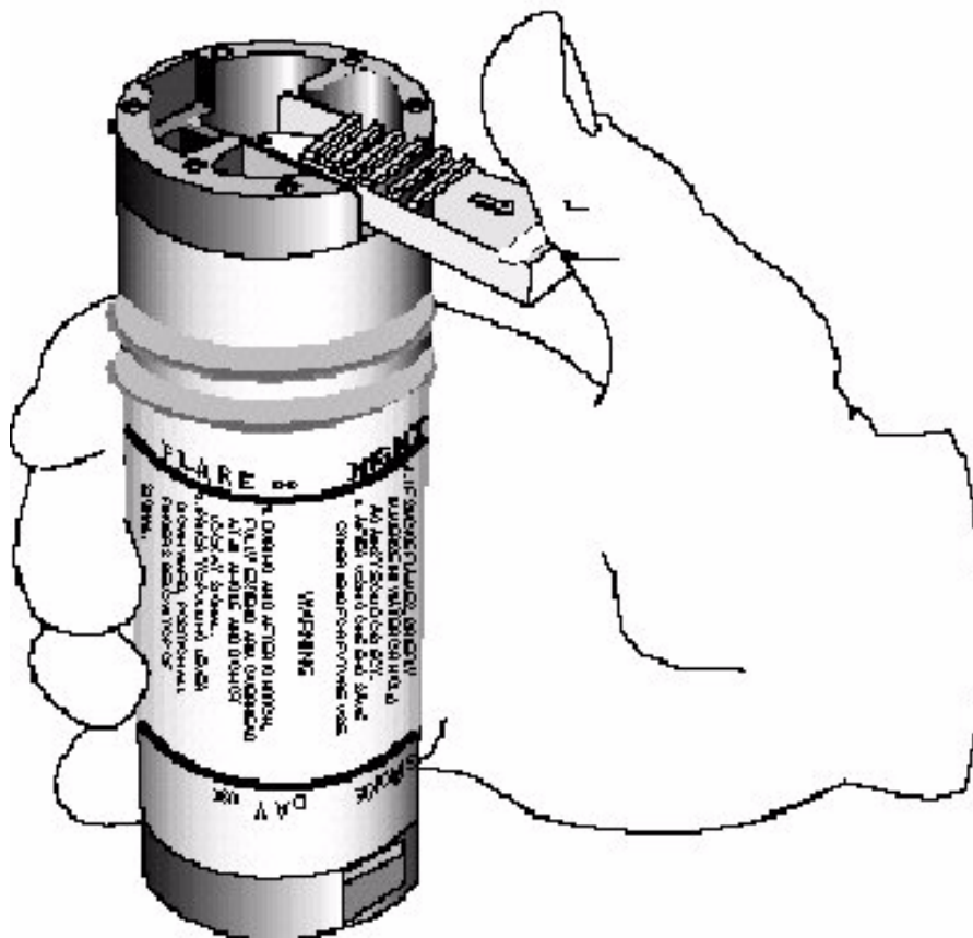
Figure 6-13 Operating the MK-124 MOD 0 Signal Flare
