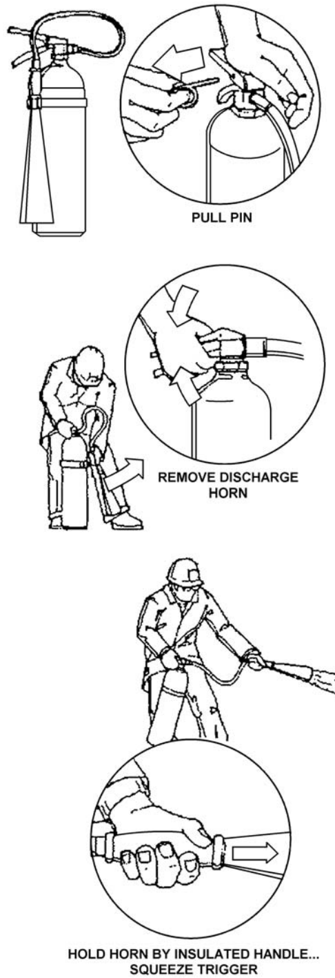
Figure 18-3 Operating the CO 2 Extinguisher
