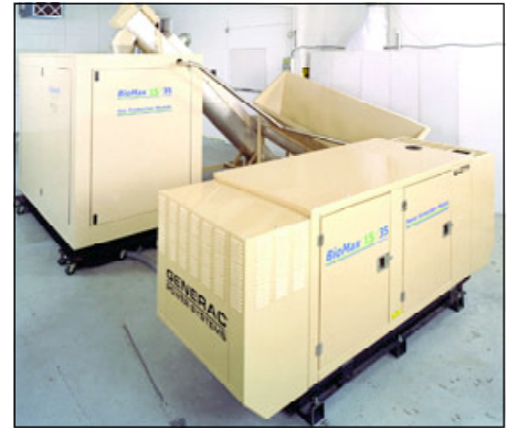
Wood gasification system for small-scale power production.
