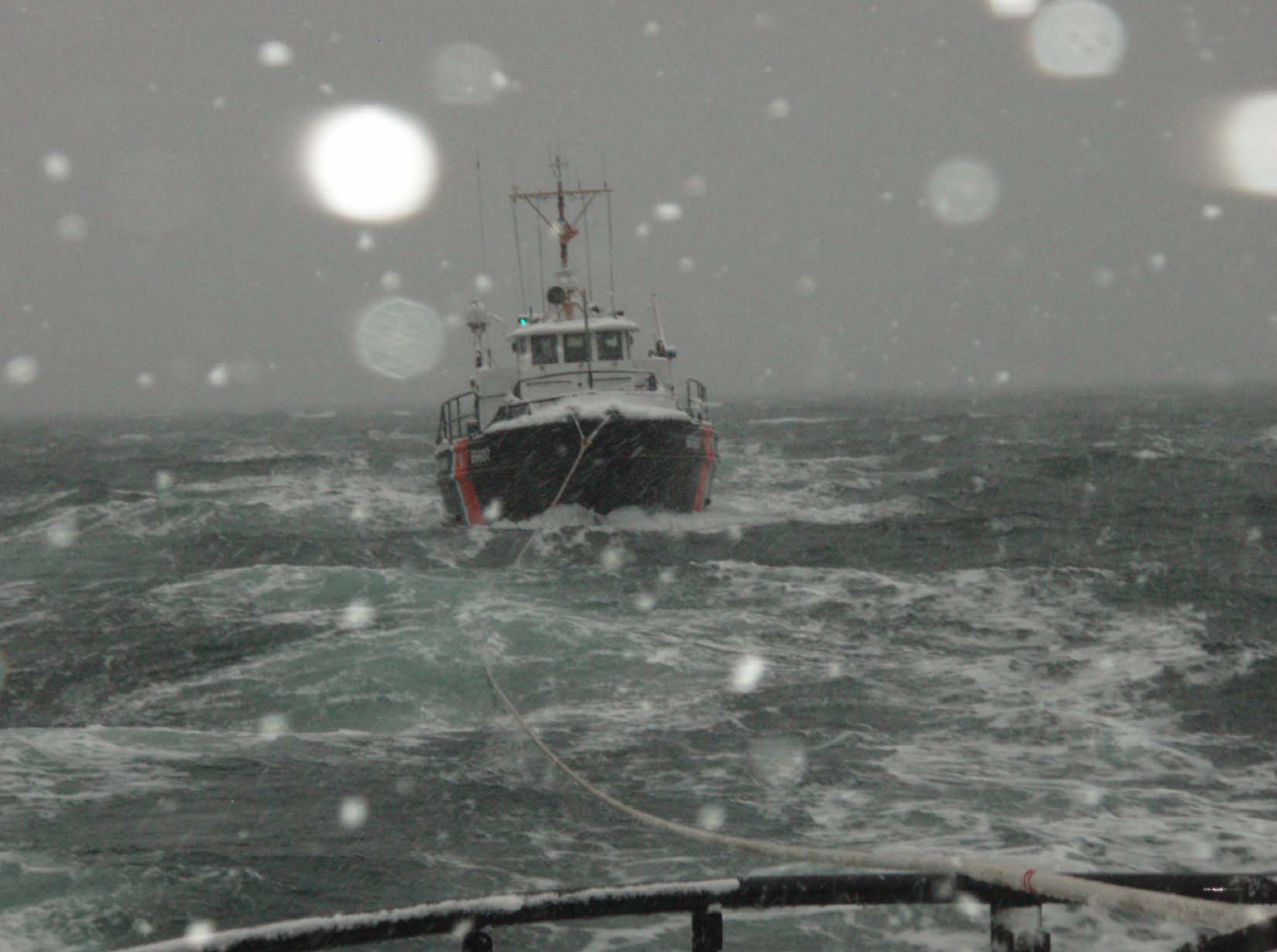
USCGC TACKLE towing USCGC BRIDLE after BRIDLE suffered a steering casualty while icebreaking on the Penobscot River. Photo by BMC Deery.
