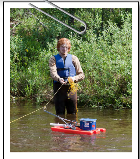
BLM Hydrology Technician Eric Deal measures stream flow on Nome Creek using an Acoustic Doppler Current Profiler (a sonar device).
