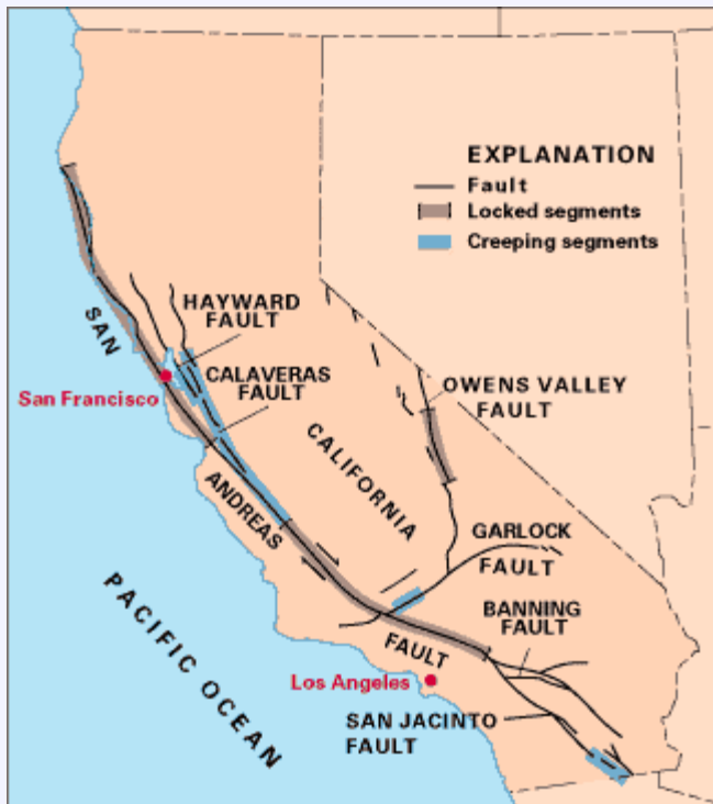
Map of the San Andreas and a few of the other faults in California, segments of which display different behavior: locked or creeping (see text). (Simplified from USGS Professional Paper 1515.)
