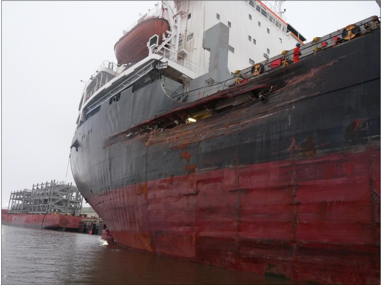
Figure 12. Damage to the Gull Arrow .
