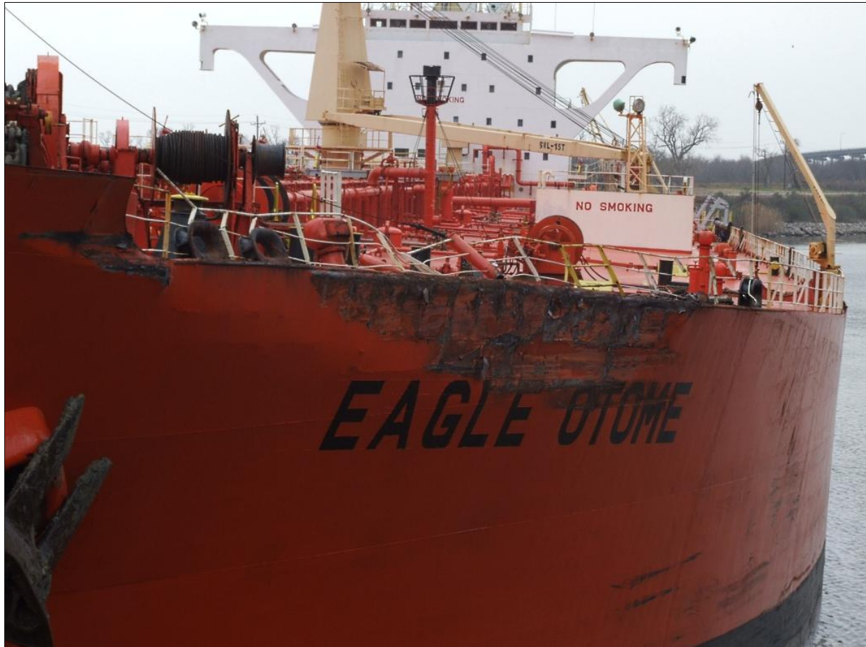
Figure 10. Portside damage to the Eagle Otome .
