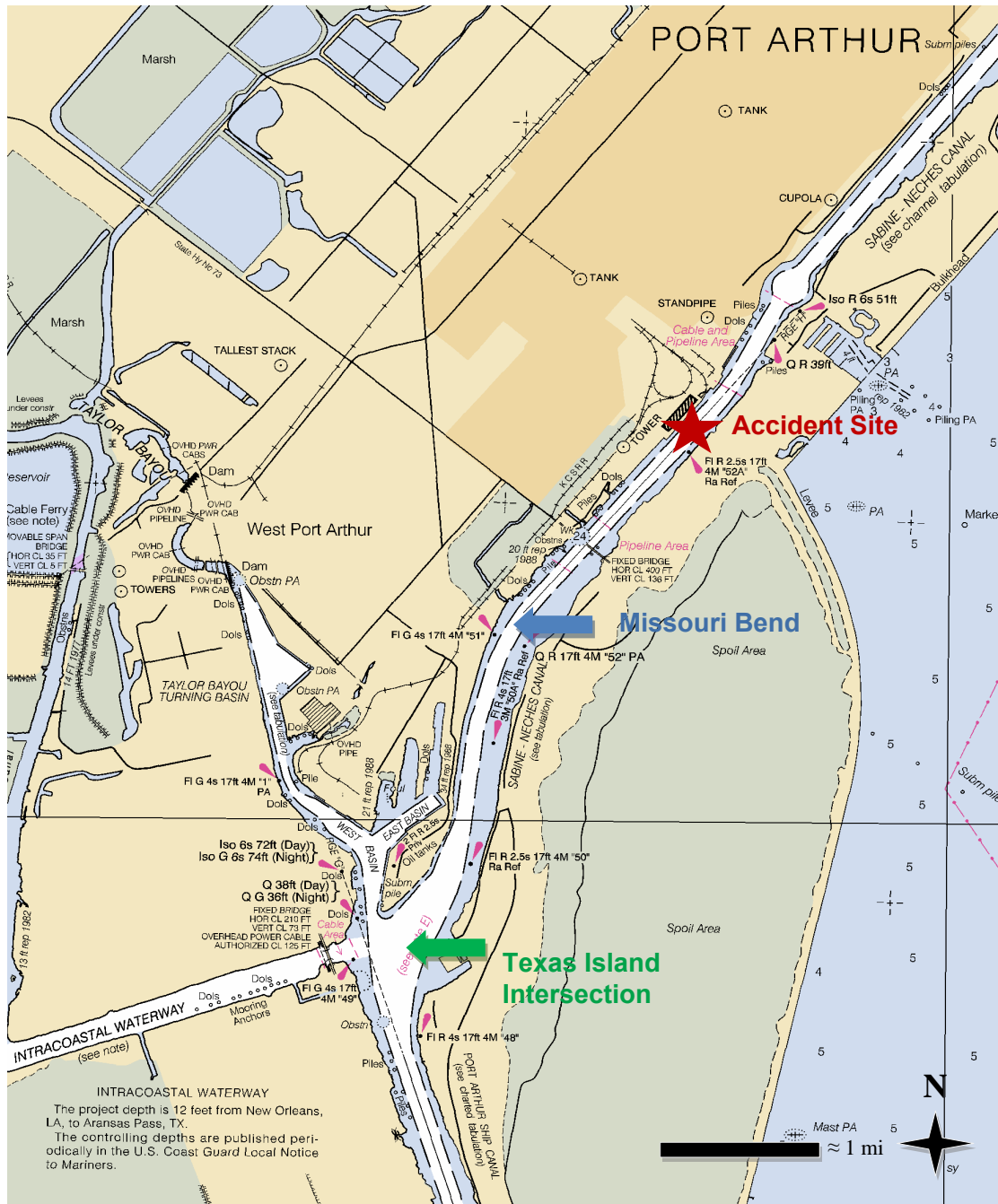
Figure 3. Section of National Oceanic and Atmospheric Administration (NOAA) chart 11342, with the Sabine-Neches Canal running north and northeast. The Texas Island Intersection is marked with a green arrow, Missouri Bend with a blue arrow, and the accident location with a red star.
