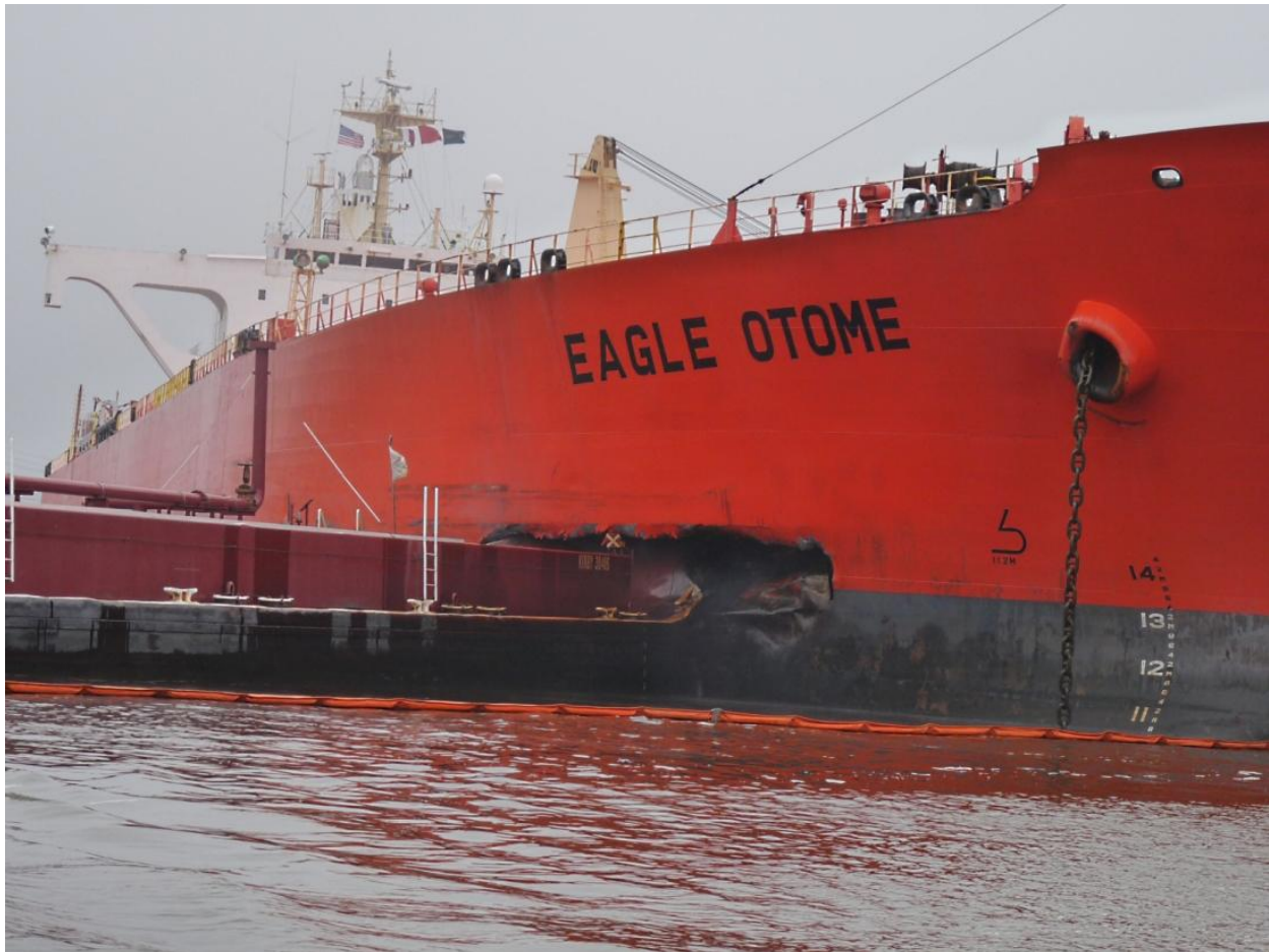
Figure 11. Starboard side of the Eagle Otome , with the Kirby 30406 lodged in it.
