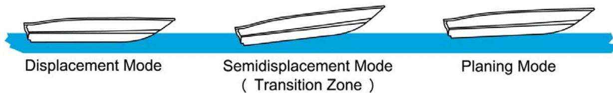
Figure 12. Stages of generic vessel planing and corresponding trim angles.
