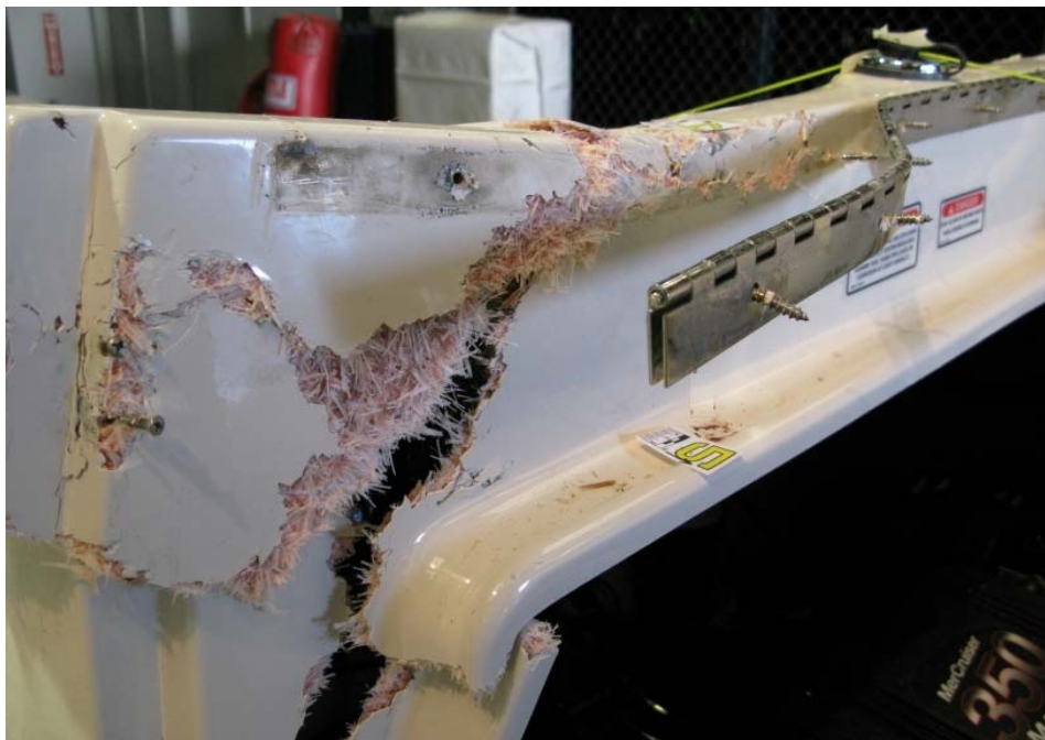
Figure 8. Fractured fiberglass on the Sea Ray, viewed looking aft and port from inside the boat's cockpit.
