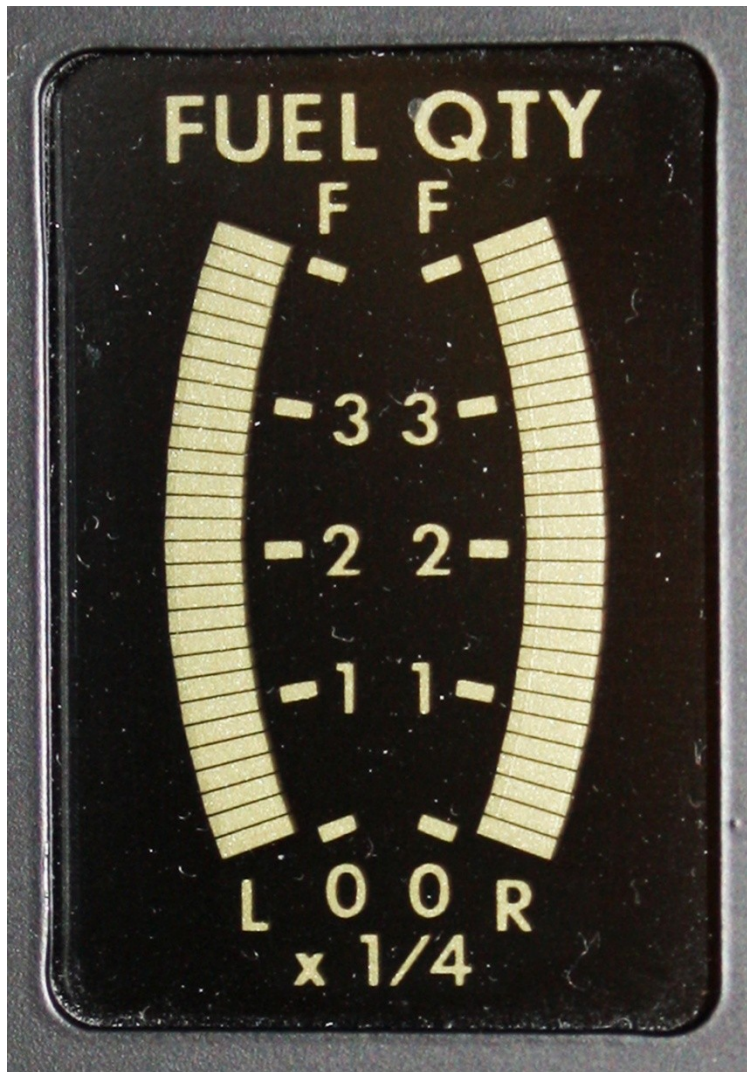
Figure 4. Fuel quantity indicator.
