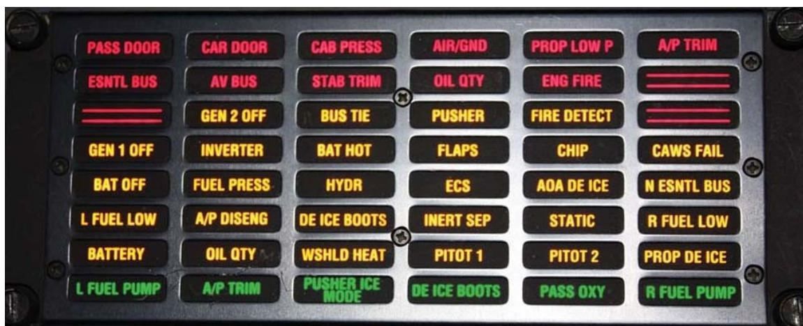
Figure 5. Central advisory and warning system display.
