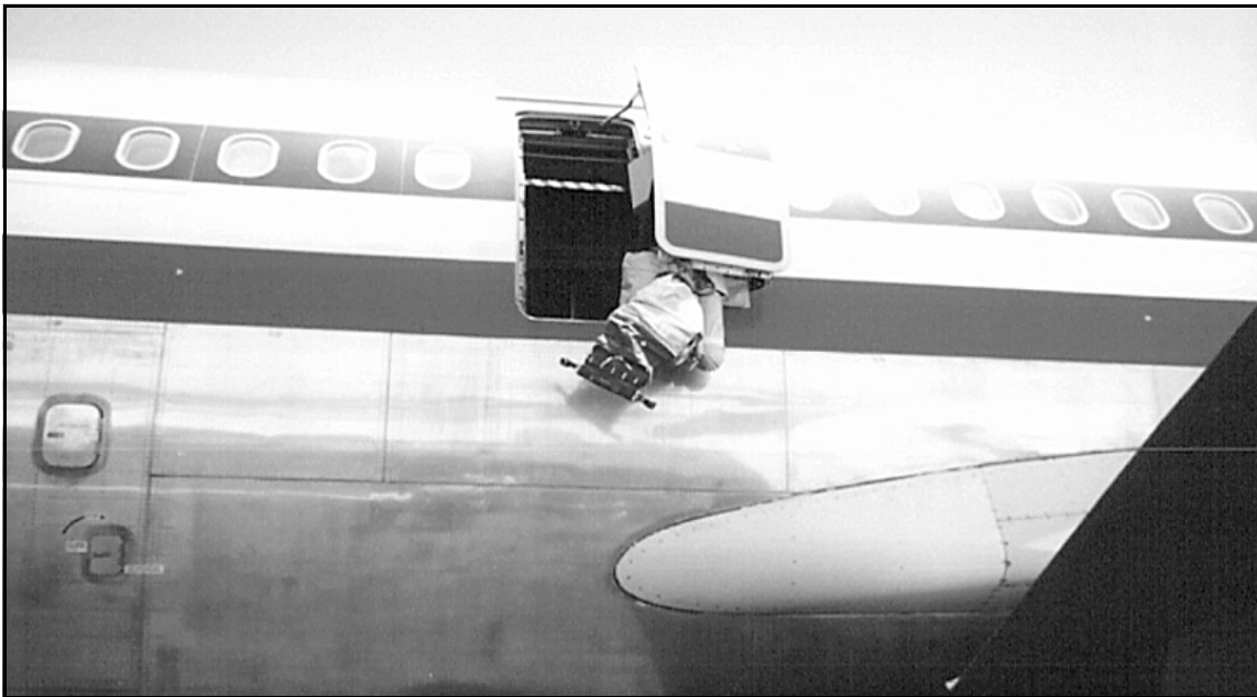
Figure 5-5. View of the R3 door that failed to operate as intended following the Airbus 300 accident on July 9, 1998, in San Juan, Puerto Rico (case 24).
