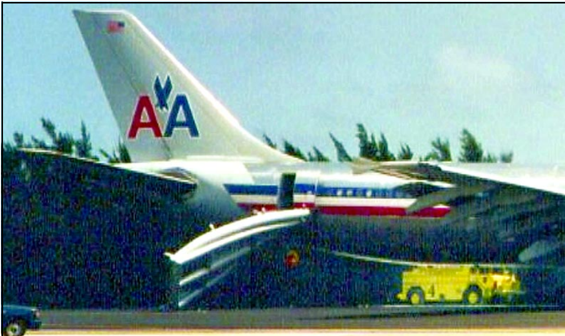
Figure 5–9. View of the wind's effect (25-knot gusts) on the evacuation slide used following the Airbus 300 accident on July 9, 1998, in San Juan, Puerto Rico (case 24). Passengers were able to use this exit after a person on the ground held the slide in place.
