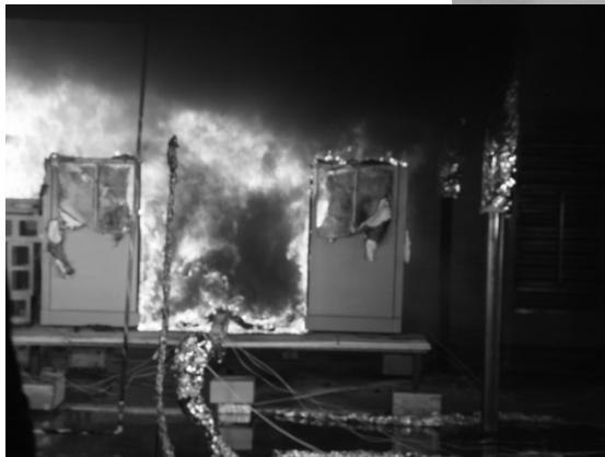
Full Involvement of Fire near Peak Heat Release Rate
