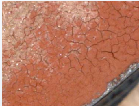
250 deg C for an hour mud cracks much more visible
