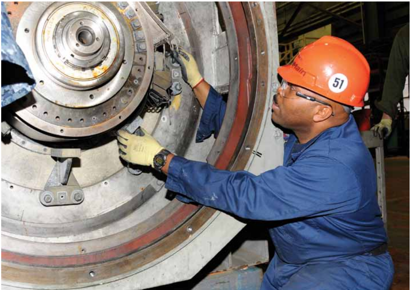
▲ Surgemain worker Electronics Technician 1st Class Errol Barbee inspects a 500 kilowatt generator in the Motor Rewind Shop in Building 240. The Surgemain Department provides mission essential services to the shipyard and is manned with U.S. Navy Reserve personnel. Portsmouth Naval Shipyard, a field activity of NAVSEA, is committed to maximizing the material readiness of the fleet. U.S. Navy photo by Jim Cleveland.
