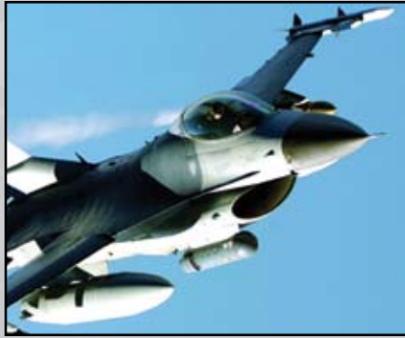
This F-16 carries a LITENING pod, an operational precision targeting pod system.
