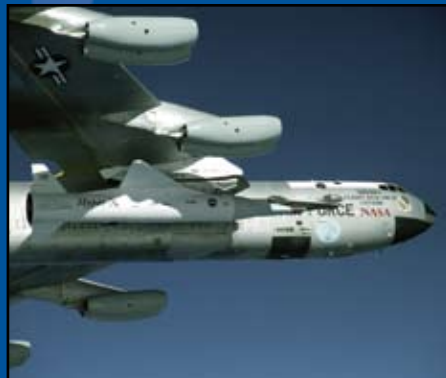
NASA's B-52 launch aircraft cruises to a test range carrying an X-43A hypersonic research aircraft attached to a Pegasus rocket.
