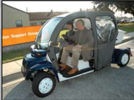
Airmen test the new Global Electric Motorcars Lackland AFB, Texas, is using to conserve energy.
