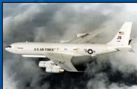
The E-8C Joint STARS is the only airborne platform in operation that can maintain realtime ground surveillance over the battlefield.
