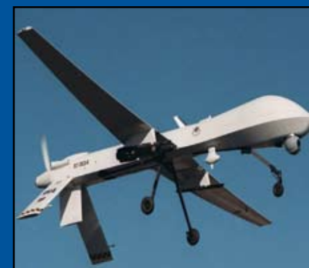
The MQ-1 Predator unmanned aerial vehicle armed with the AGM-114 Hellfire missile.
