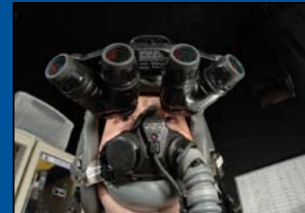
An Airman performs an operational check of panoramic night vision goggles. The devices give pilots a 90-degree field of view.
