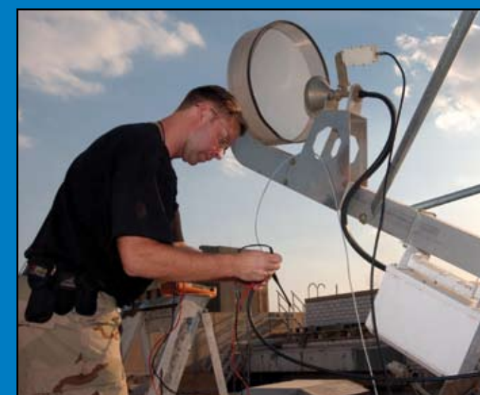
An Airman calibrates a satellite communications ground station in Iraq.
