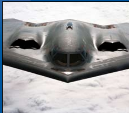
The B-2's composite materials, special coatings and flying-wing design all contribute to its "stealthiness."
