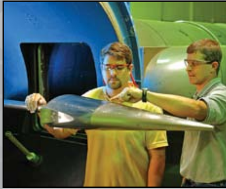
Test engineers ready a Hypersonic Technology Vehicle-1 model.
