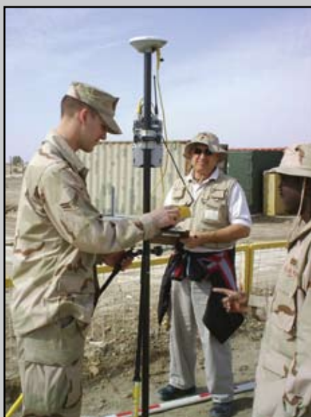
Air Force and Army civil engineers monitor a sensor used to gather information from a Global Positioning System satellite.
