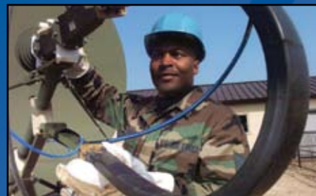
A maintenance technician sets up a mobile tactical super-high frequency satellite communications terminal.
