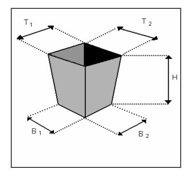
Calculate top (Y) and bottom (Z) area in square inches using  $T_1$ ,  $T_2$ ,  $B_1$ , and  $B_2$  in inches:
