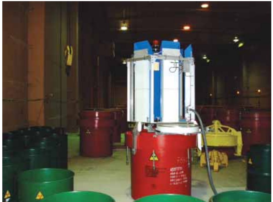
STRENGTHENING SAFEGUARDS: International Nuclear Safeguards Engagement Program-developed Chornobyl Drum Assay System during acceptance tests at the Chornobyl Nuclear Power Plant.
