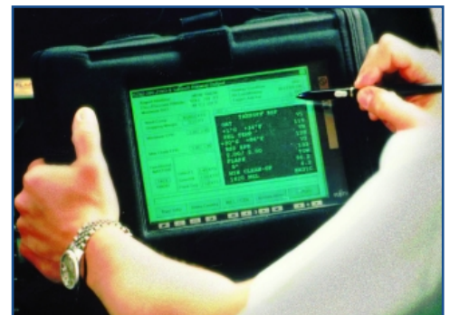
Electronic Flight Bags. Instead of traditional flight bags loaded with paper documents such as checklists, operating manuals, and navigation publications, many flight crews are bringing aboard electronic flight bags (EFBs) in the form of handheld, laptop, or tablet computers, as shown above. In support of FAA, the Volpe Center has performed significant research related to EFBs and has developed guidelines for their design and evaluation. Details on the Center's EFB work are available at www.volpe.dot.gov/opsad/efb . (Photo courtesy of Teledyne Controls)
