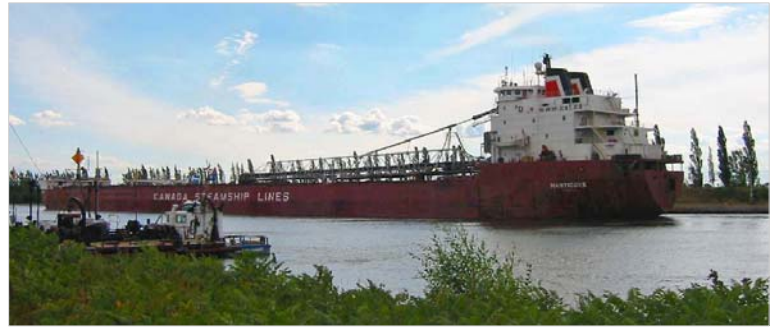
The Nanticoke, shown here passing through the Saint Lawrence Seaway, is a self-unloader bulk carrier owned and operated by Canadian Steamship Lines (CSL). The vessel trades on the Great Lakes – St. Lawrence Seaway system. (Volpe Center Photo)
