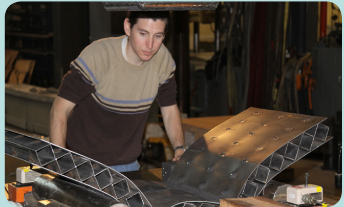
Michael Carolan, mechanical engineer at the Volpe Center, inspects a prototype panel after a structural bend test at the Lehigh Center for Advanced Technology for Large Structural Systems.
