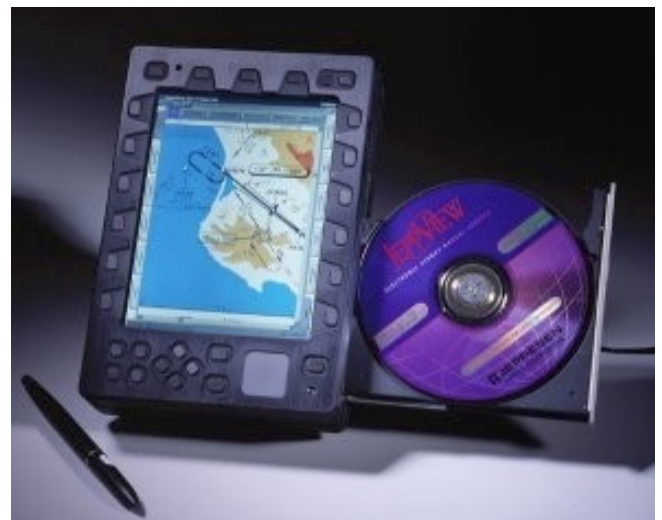
Electronic Flight Bags are portable electronic devices that can be customized to support flight deck tasks.
