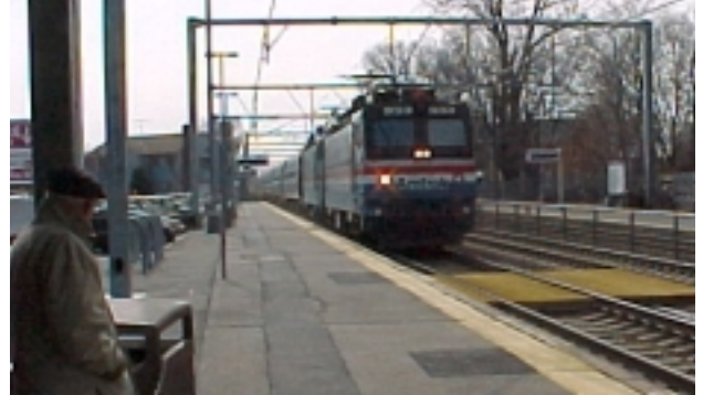
The TAMS field test began as the electric high-speed Amtrak Acela Regional Service train approached the MBTA Hyde Park station at 110 mph.
