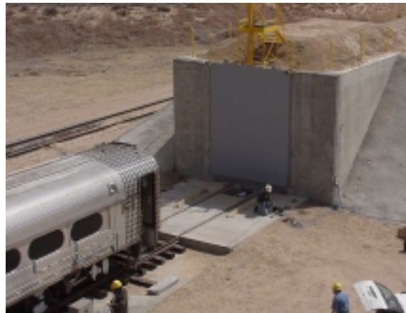
The full-scale crash test on April 4, 2000, involved two coupled commuter railcars traveling at 26 mph and colliding head on with a concrete wall.
