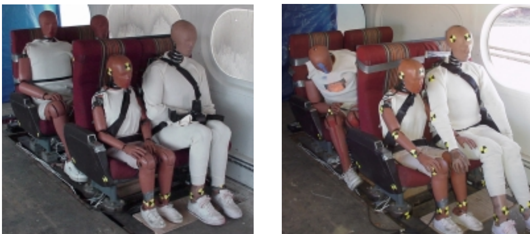
Instrumented Hybrid II and Hybrid III dummies were used to measure the injury hazard conditions to passengers inside the railcars.
