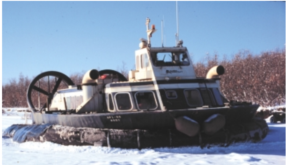
The British Hovercraft Corporation Model AP1-88 air cushion vehicle delivers U.S. mail to remote villages in Alaska.
